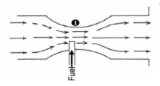
A venturi is a constriction of the inside diameter of a tube. The "venturi affect" occurs when airflows through a constriction, the airflow speeds up (velocity increases) and the pressure decreases (vacuum increases) at the point of the smallest diameter.
