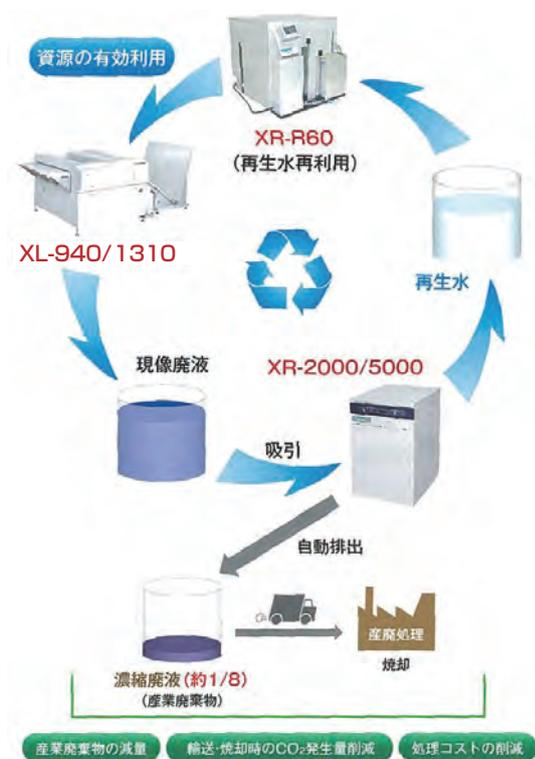
Fig. 8 Systematic view of reducing waste developer/rinse water.
