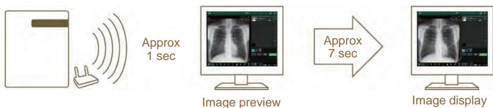
Fig. 7 FDR D-EVO plus C24i/s exposure cycle time.
