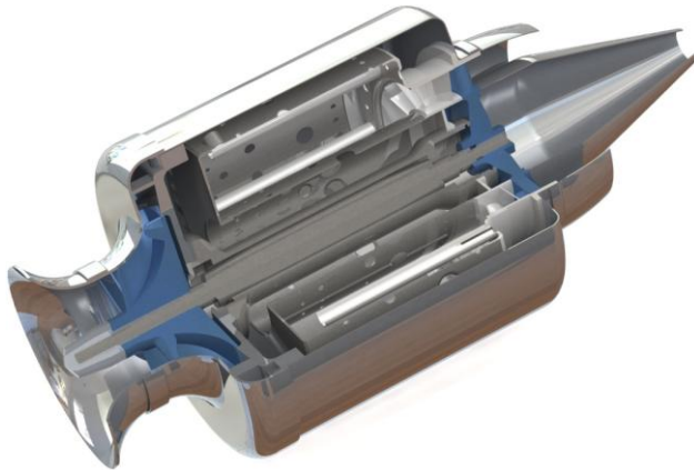
Figure 2. The model of KJ 66 engine in FloEFD.
