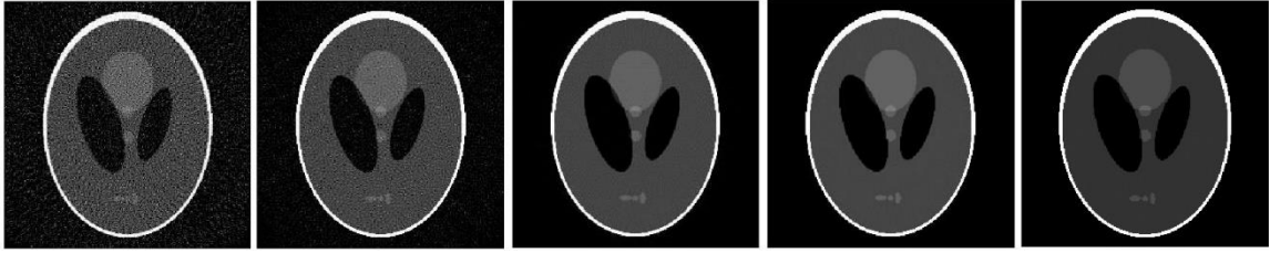
Figure 3.8 Left to right: SheppLogan phantom reconstruction result using Wavelet, Curvelet, TV, CTV, and the Nonconvex L1-L2 methods
