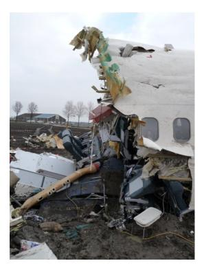
All major items of the aircraft were accounted for, and there was no evidence of in-flight breakup. A significant quantity of fuel was found in both main fuel tanks and there was no evidence of any rupture of the tanks. There was no evidence of an in-flight explosion. There was no sign of fire.
