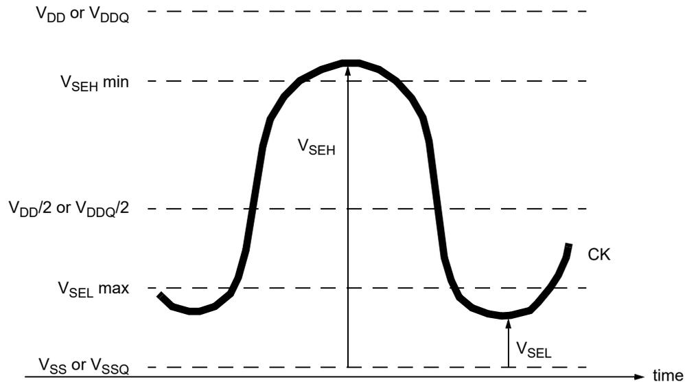
**Figure 191 — Single-ended requirement for differential signals.**
