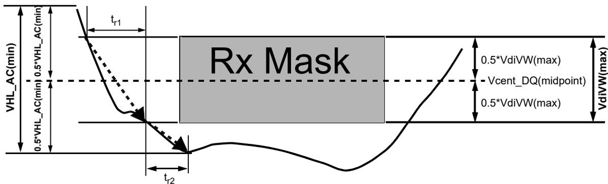
Figure 215 — Slew Rate Conditions For Falling Transition
