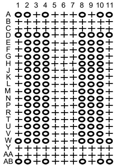
Figure 2 — DDR4 Ball Assignments for the x16 component
