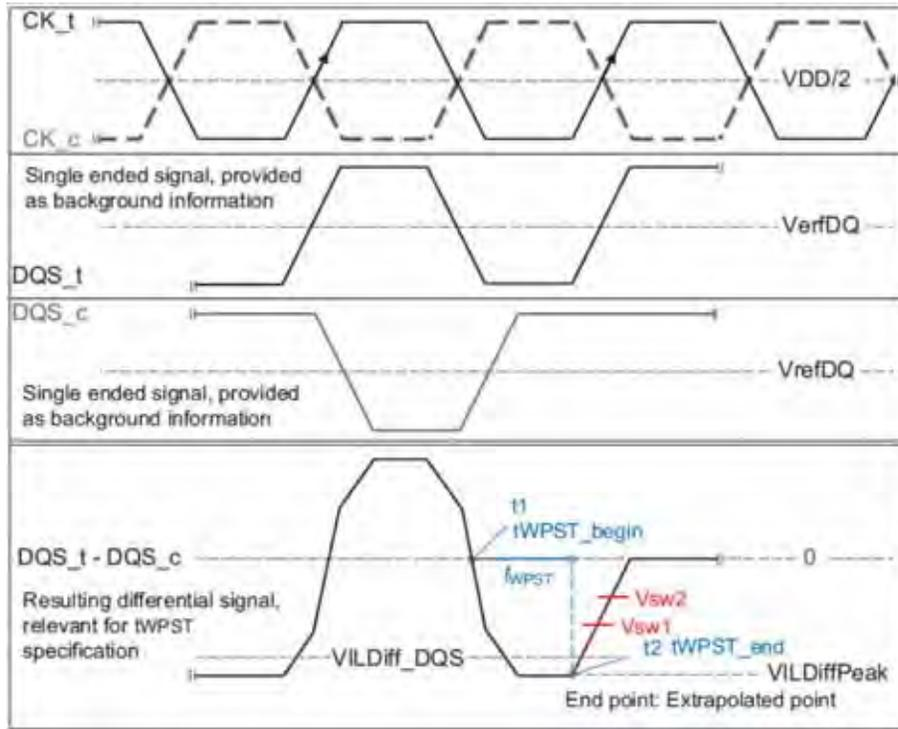
Figure 113 — Method for calculating tWPST transitions and endpoints
