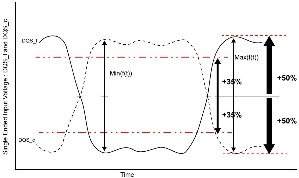
Figure 200 — Definition of differential DQS Peak Voltage and range of exempt nonmonotonic signaling
