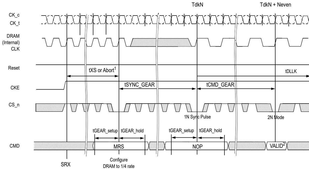
NOTE 1 CKE High Assert to Gear Down Enable Time (tXS, tXS\_Abort) depend on MR setting. A correspondence of tXS/tXS\_Abort and MR Setting is as follows.
