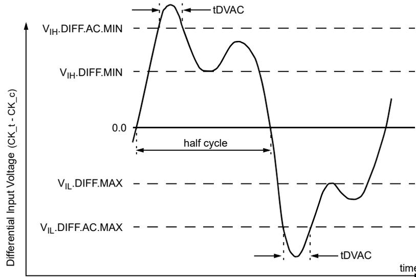
NOTE 1. Differential signal rising edge from  $V_{IL.DIFF.MAX}$  to  $V_{IH.DIFF.MIN}$  must be monotonic slope.
