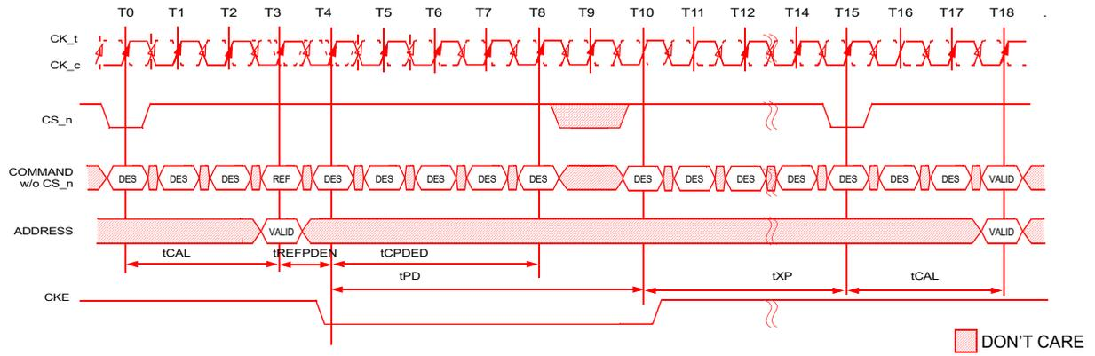
**Figure 46 — Refresh Command to Power Down Entry**
