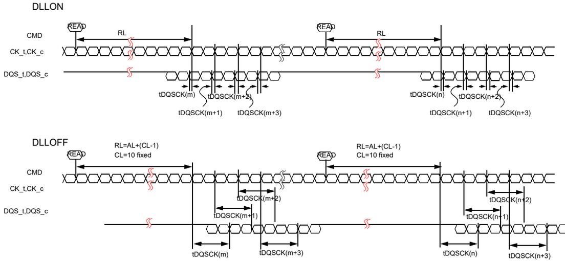
Figure 168 — tDQSK Definition Difference between DLL ON and DLL OFF
