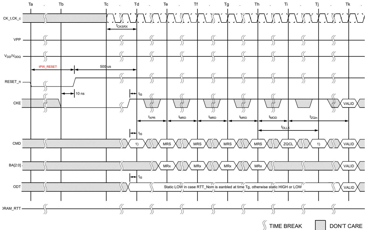
NOTE 1 From time point 'Td' until 'Tk', DES commands must be applied between MRS and ZQCL commands
