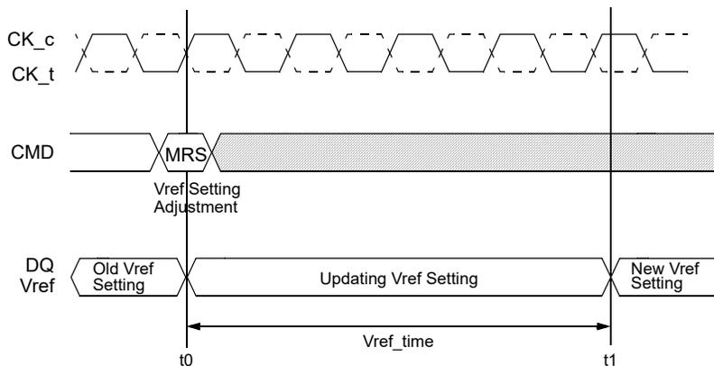
**Figure 29 — Vref\_time timing diagram**
