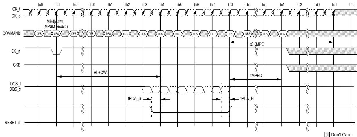
Figure 161 — Maximum Power Saving mode Entry with PDA
