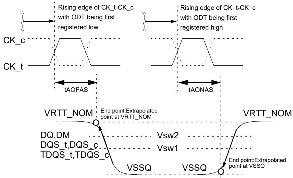
**Figure 188 — Definition of  $t_{AOFAS}$  and  $t_{AONAS}$**
