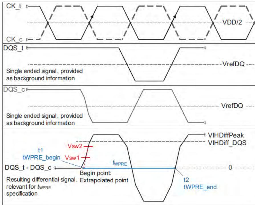
Figure 112 — Method for calculating tWPRE transitions and endpoints
