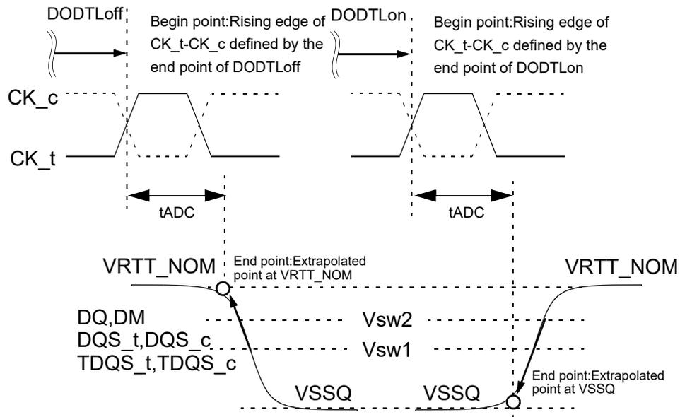
**Figure 186 — Definition of  $t_{ADC}$  at Direct ODT Control**
