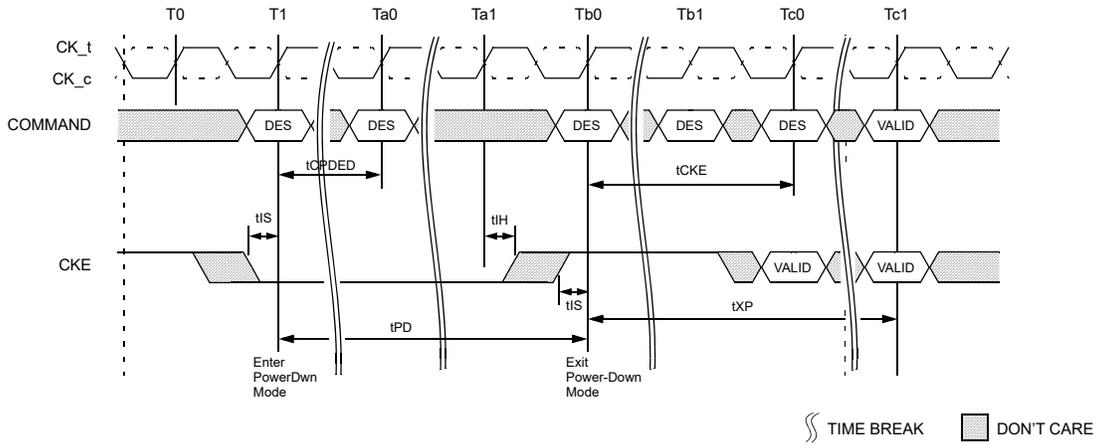
Figure 153 — Precharge Power-Down Entry and Exit
