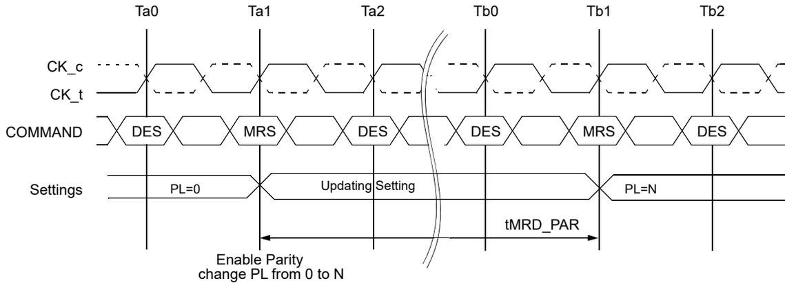
NOTE 1  $tMRD\_PAR = tMOD + N$ ; where N is the programmed parity latency with the MRS command entering CA parity mode.
