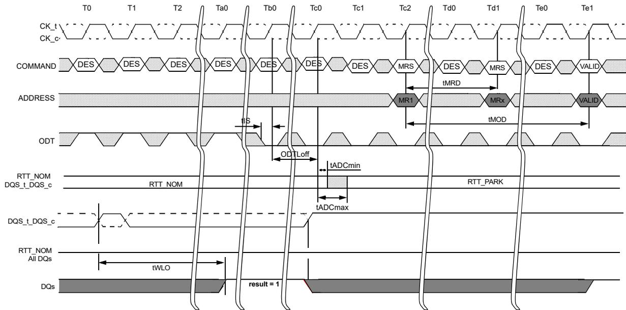
Figure 16 — Timing details of Write leveling exit
