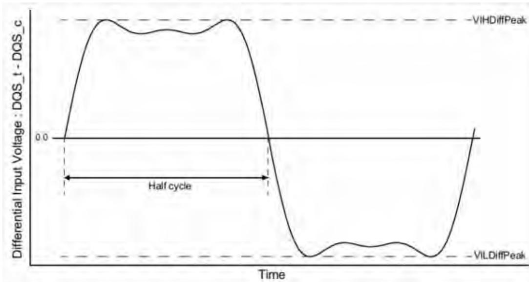
Figure 199 — Definition of differential DQS Signal AC-swing Level
