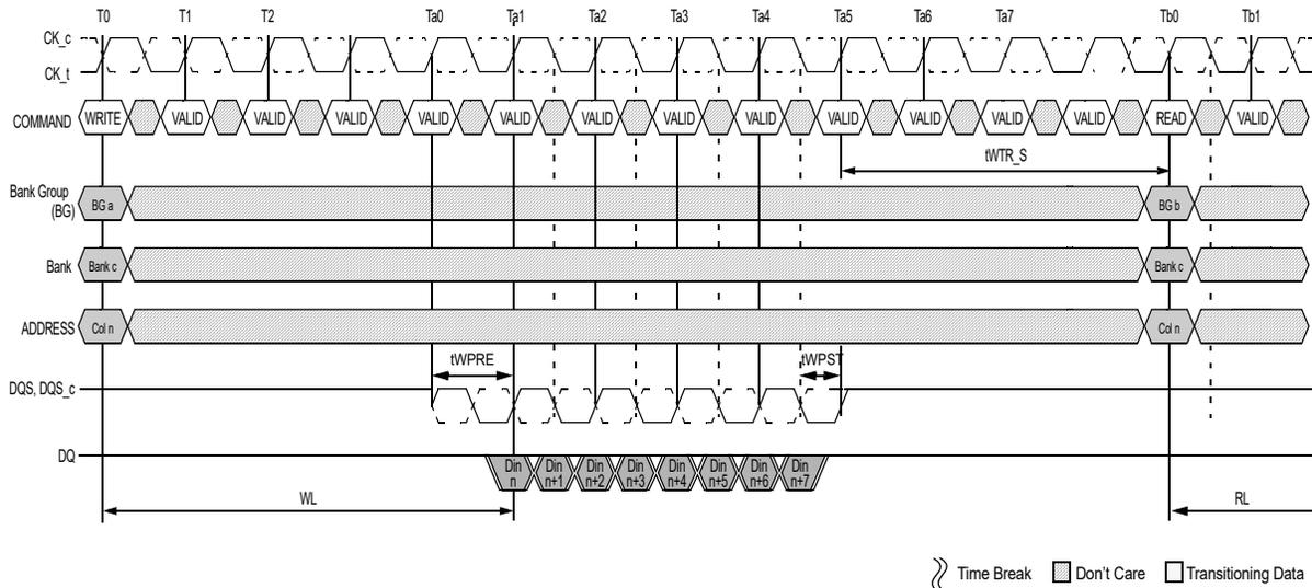
NOTE 1 tWTR\_S : Delay from start of internal write transaction to internal read command to a different Bank Group. When AL is non-zero, the external read command at Tb0 can be pulled in by AL.
