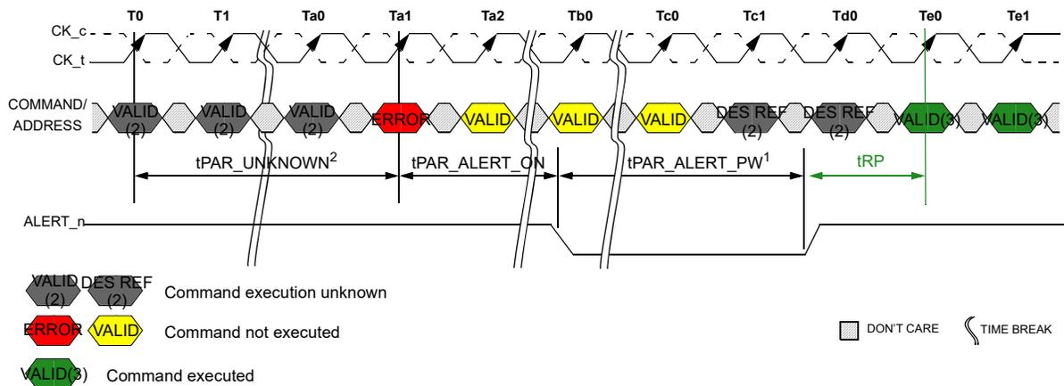
NOTE 1 DRAM is emptying queues, Precharge All and parity checking off until Parity Error Status bit cleared.
