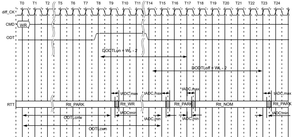
$\text{ODT}_{\text{cnw}} = \text{WL} - 2$  (1tCK preamble),  $\text{WL} - 3$  (2tCK preamble)
