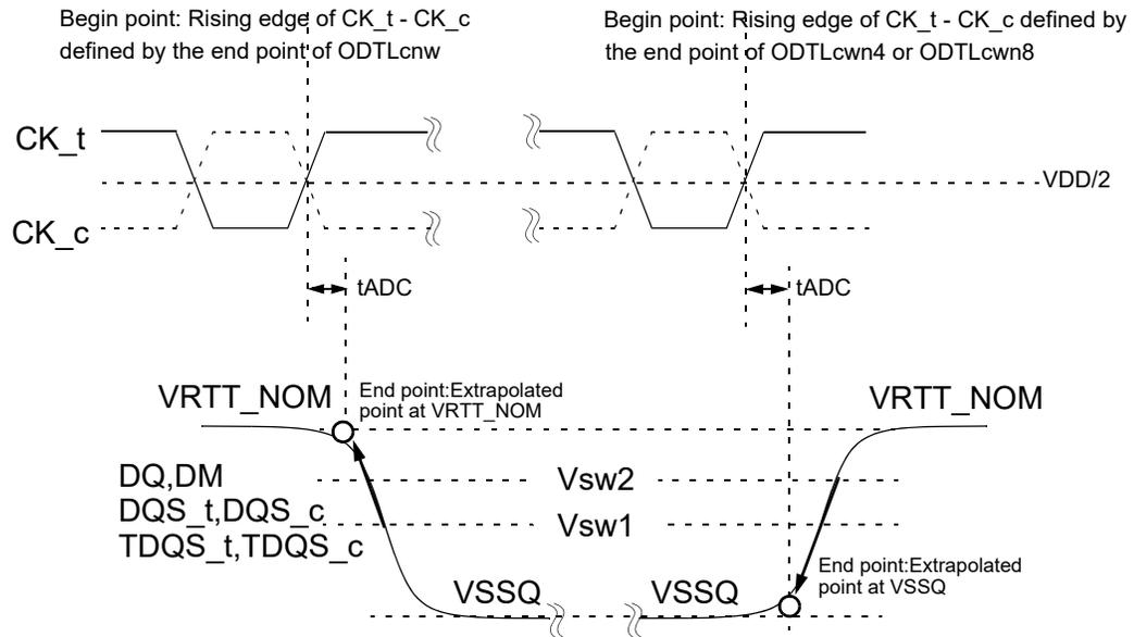
**Figure 187 — Definition of  $t_{ADC}$  at Dynamic ODT Control**
