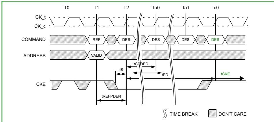
Figure 154 — Refresh Command to Power-Down Entry
