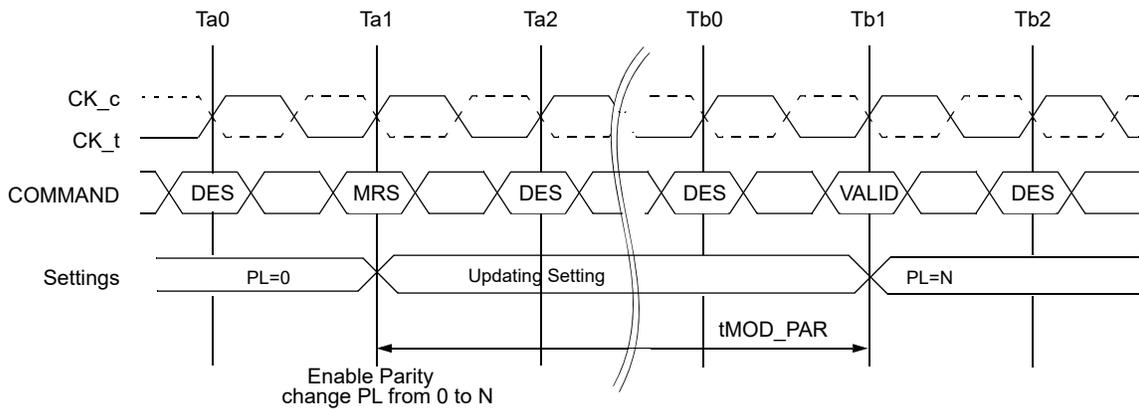
NOTE 1  $tMOD\_PAR = tMOD + N$ ; where N is the programmed parity latency with the MRS command entering CA parity mode.
