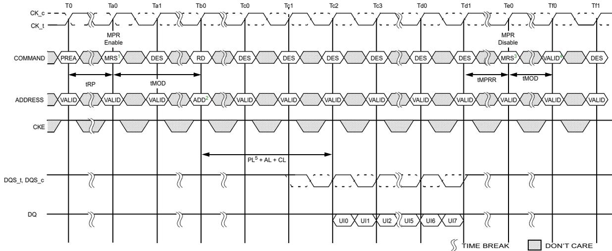
NOTE 1 Multi-Purpose Registers Read/Write Enable (MR3 A2 = 1)
