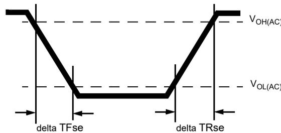
**Figure 204 — Single-ended Output Slew Rate Definition**
