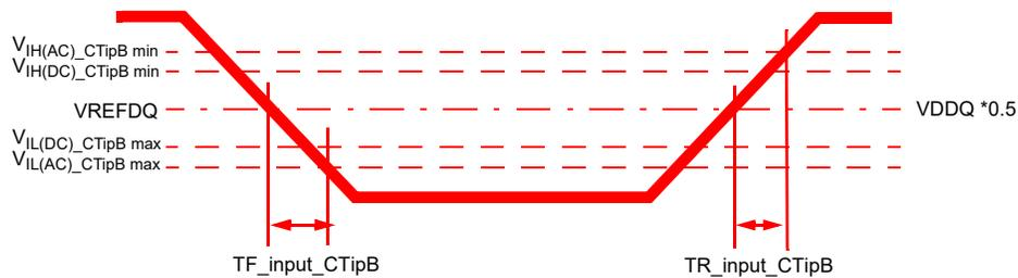
**Figure 167 — Input B Slew Rate Definition**
