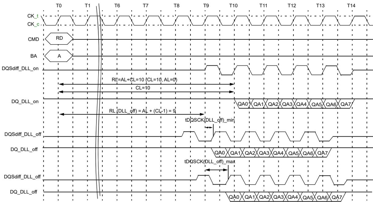
Figure 13 — READ operation at DLL-off mode
