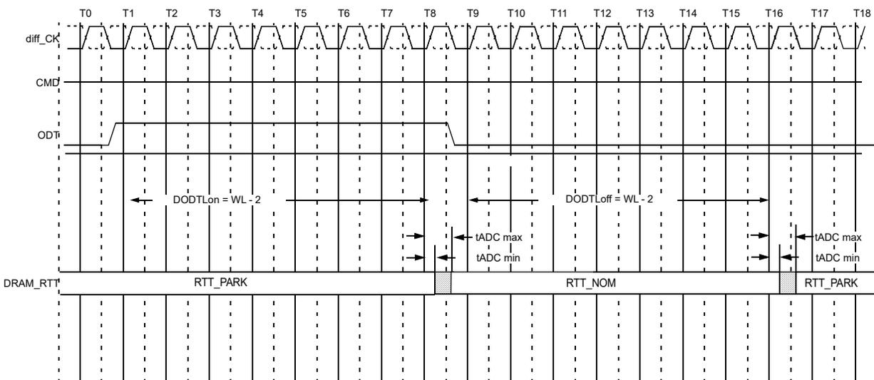
**Figure 176 — Synchronous ODT Timing Example for CWL=9, AL=0, PL=0; DODTLon=WL-2=7; DODTLoff=WL-2=7**
