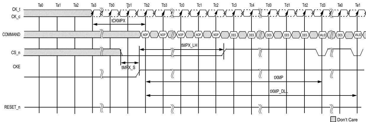
Figure 163 — Maximum Power Saving Mode Exit Sequence
