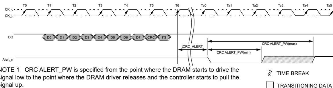
NOTE 1 CRC\_ALERT\_PW is specified from the point where the DRAM starts to drive the signal low to the point where the DRAM driver releases and the controller starts to pull the signal up.
