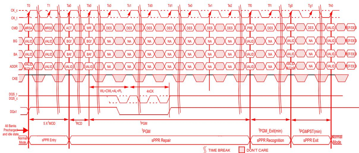
**Figure 173 — Fail Row Soft PPR (WR Case)**
