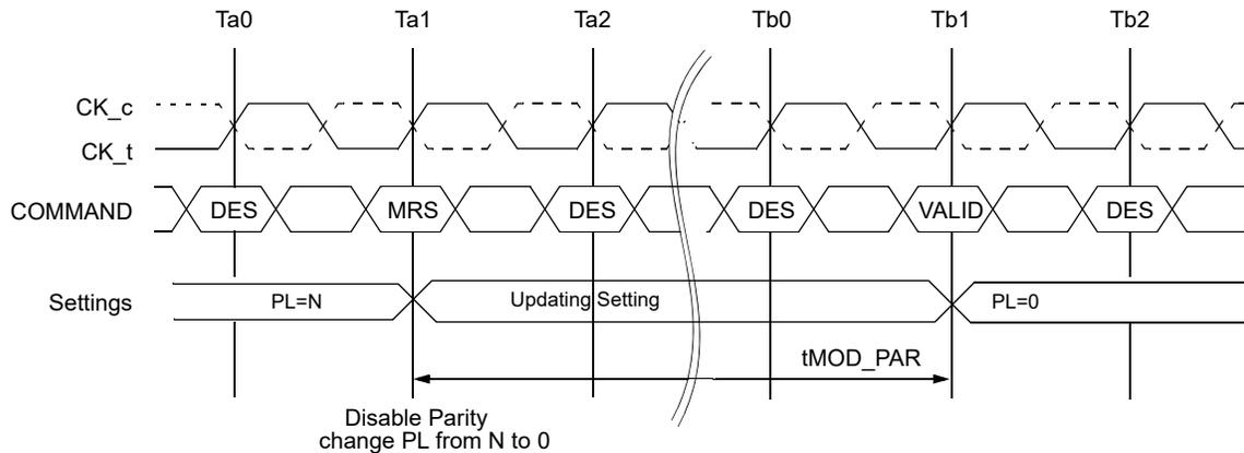
NOTE 1  $tMOD\_PAR = tMOD + N$ ; where N is the programmed parity latency prior to the MRS command exiting CA parity mode.
