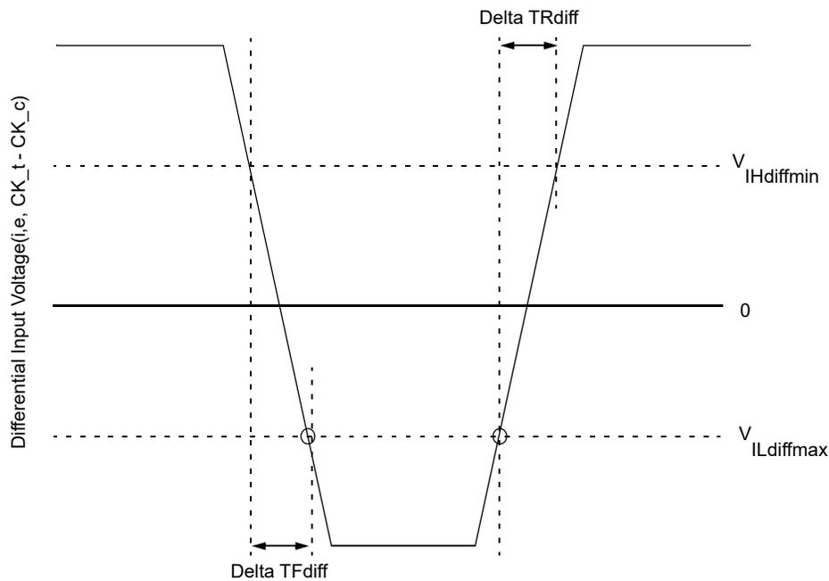
**Figure 195 — Differential Input Slew Rate Definition for CK<sub>t</sub>, CK<sub>c</sub>**
