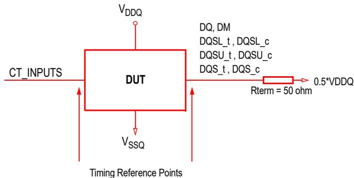
**Figure 207 — Connectivity Test Mode Timing Reference Load**
