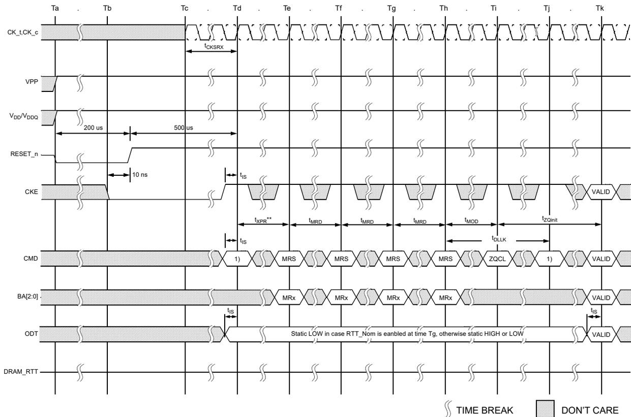
NOTE 1 From time point 'Td' until 'Tk', DES commands must be applied between MRS and ZQCL commands.
