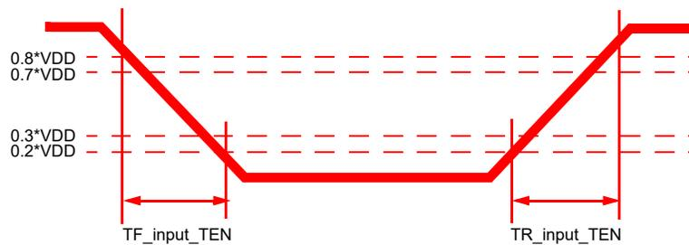
**Figure 165 — TEN Input Slew Rate Definition**
