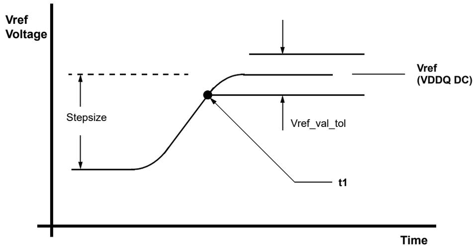
Figure 31 — Vref step single stepsize increment case
