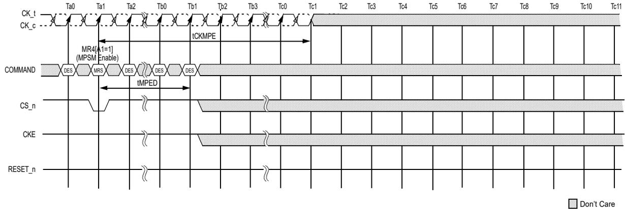
Figure 160 — Maximum Power Saving mode Entry
