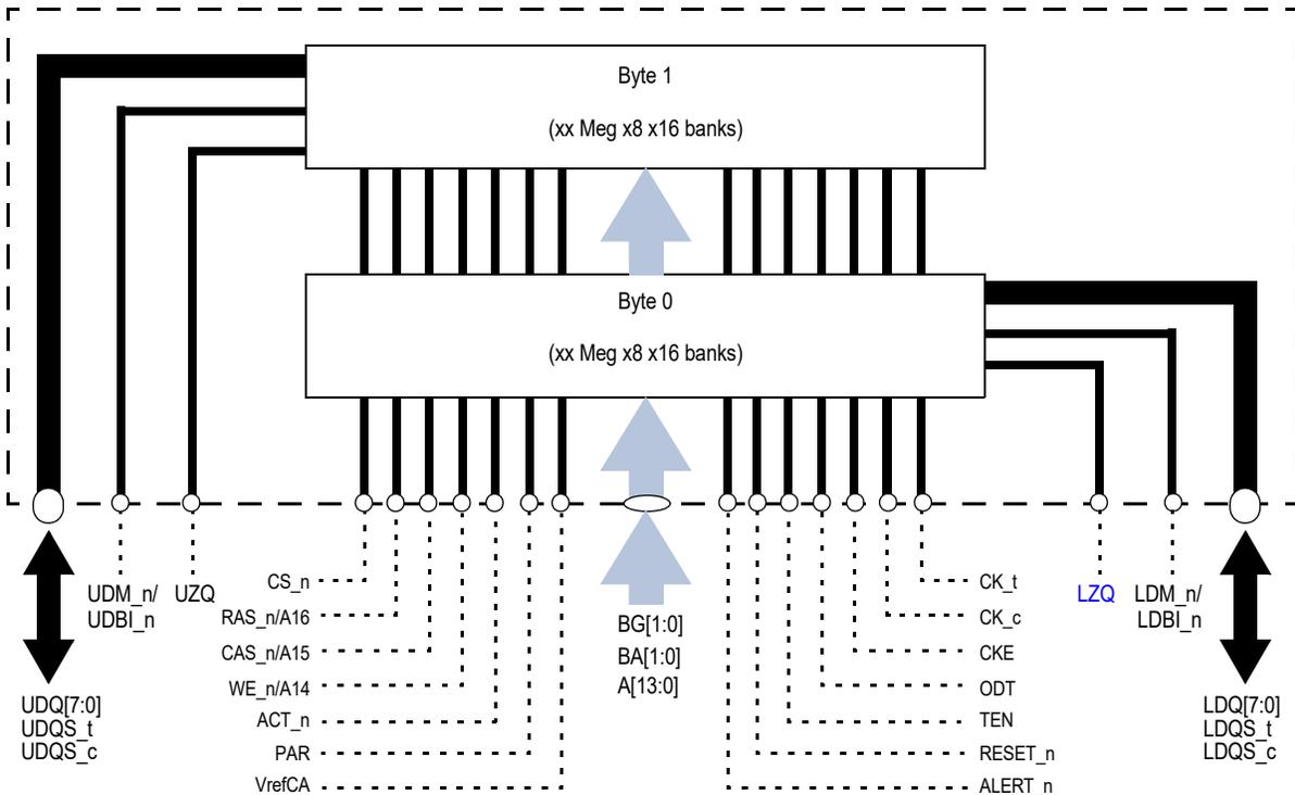
Figure 4 — Functional Block Diagram of SR x16 DDP
