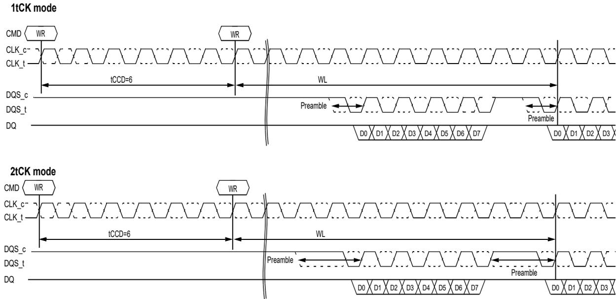
Figure 68 — t<sub>CCD</sub>=6 (AL=PL=0)
