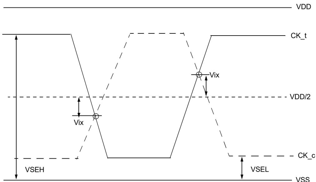
Figure 197 —  $V_{ix}$  Definition (CK)
