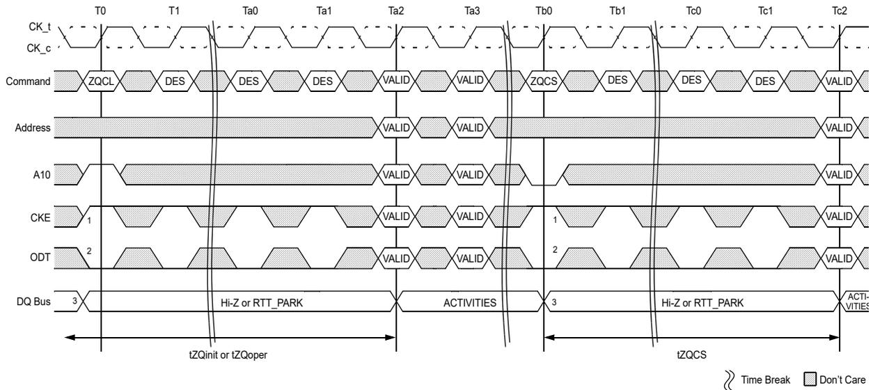
NOTE 1 CKE must be continuously registered high during the calibration procedure.
