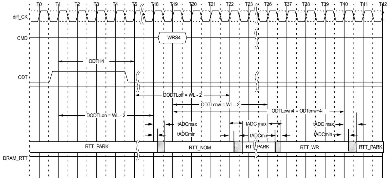
**Figure 177 — Synchronous ODT example with BL=4, CWL=9, AL=10, PL=0; DODT<sub>Lon/off</sub>=WL-2=17, ODT<sub>cnw</sub>=WL-2=17**
