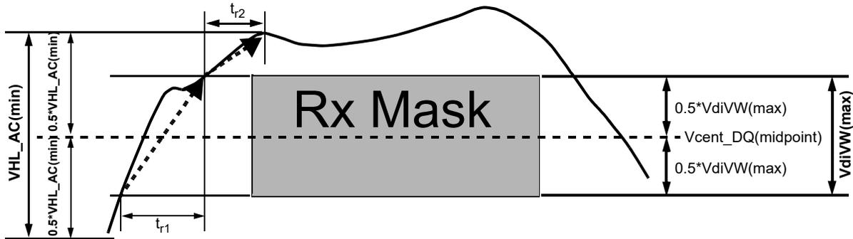
Figure 214 — Slew Rate Conditions For Rising Transition
