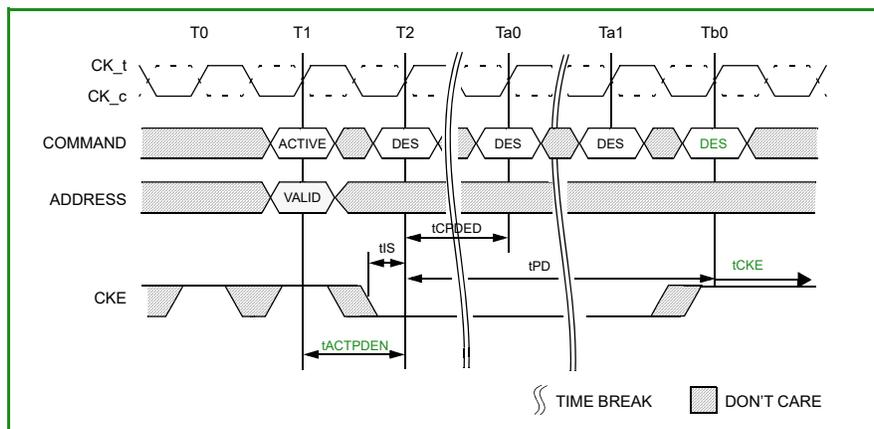
Figure 155 — Activate Command to Power-Down Entry
