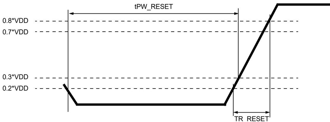
**Figure 198 — RESET\_n Input Slew Rate Definition**
