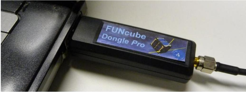
*Figure 1 FUNcube Dongle Software Defined Radio*
