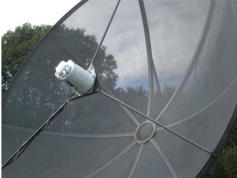
Figure 7 3m diameter dish with waveguide feed
