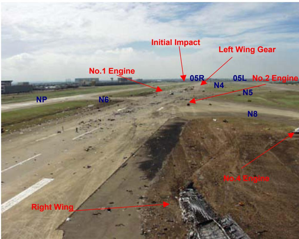
Figure 1.12-4 Wreckage distribution as seen opposite from the flight path
