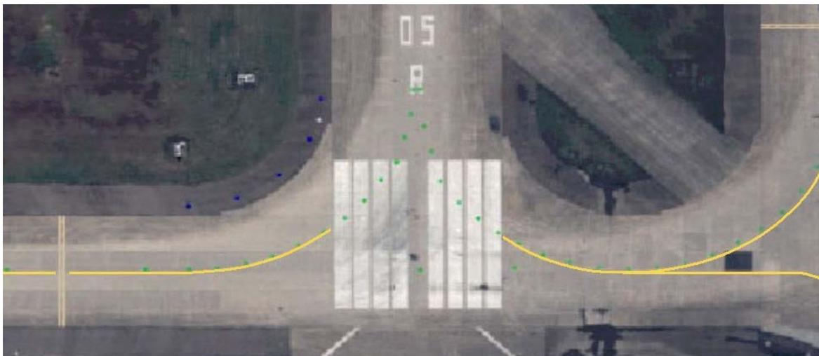
**Figure 1.10-6 Taxiway centerline marking near the threshold areas of Runway 05R**
