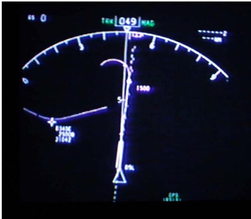
Figure 1.18-4 The display of the ND when the aircraft was lined up on Runway 05R
