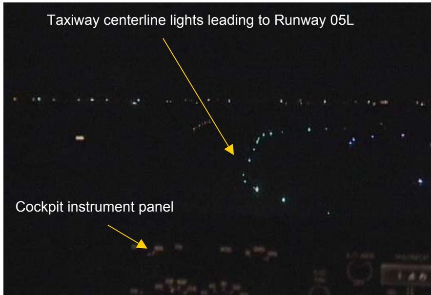
**Figure 1.16-1 Taxiway centerline lights leading to Runway 05L (field of view from Boeing 747-400 cockpit-captain side)**
