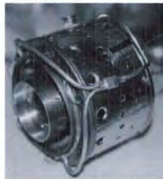
Chamber above showing early fuel pipe arrangement
