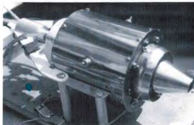
MW54 mounted on thrust-test trolley complete with electric starter
