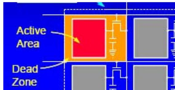
**Fig 6. The Concept of Fill Factor**
