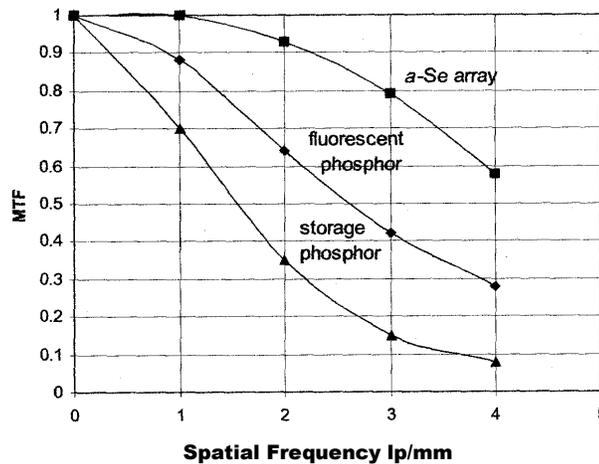
**Fig 8. Comparison of MTF of different imaging devices**
