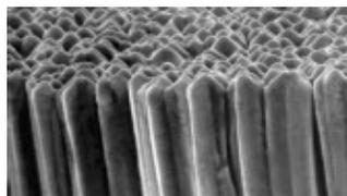
*Fig 4. Scintillation crystals grown in needle shape*
