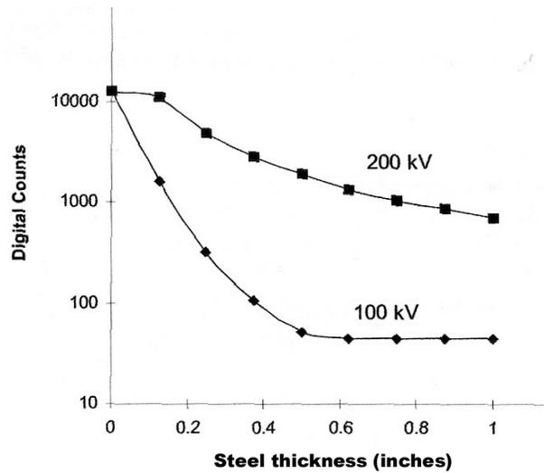
**Fig 7(b). Subject Contrast in Steel using  $\alpha$ -Se detector**
