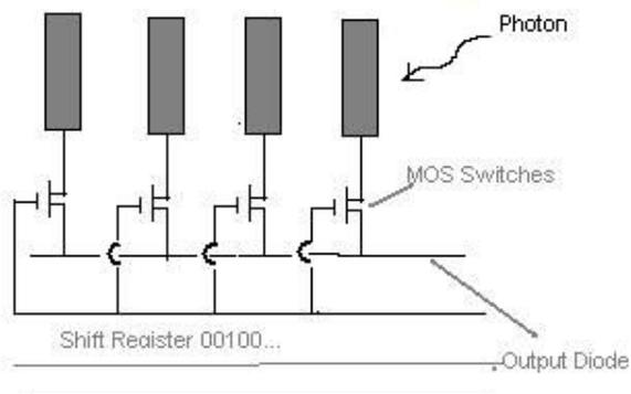
**Fig 1. Typical construction of the photodiode array**
