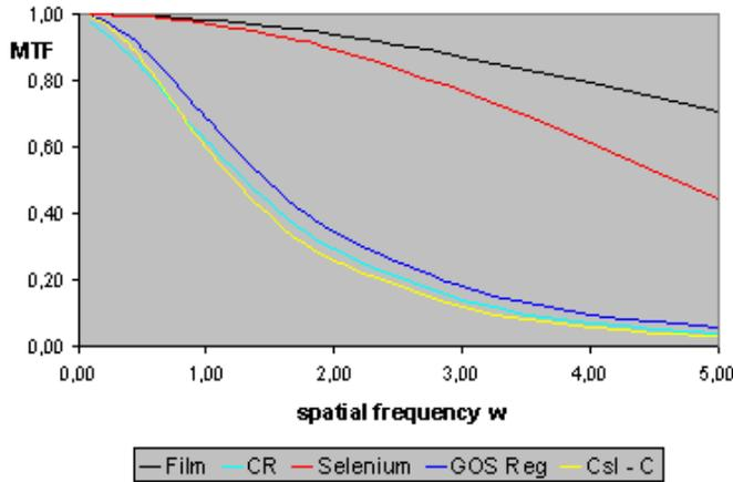
**Fig 9(a).** Comparison of MTF of Film ,CR and DR systems at 100kV x-ray energy
