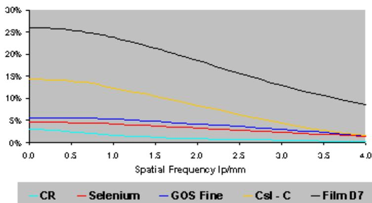
Fig 10(a). DQE(w) for various detectors and film
