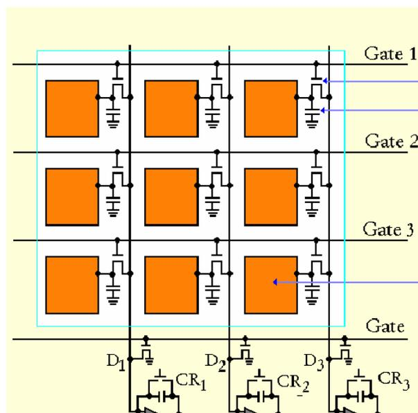
**Fig 2. A small segment of Flat Panel Detector showing pixel layout**
