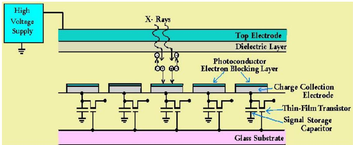
**Fig.5 Structure of Direct type FPD using photoconductor layer of amorphous Selenium**
