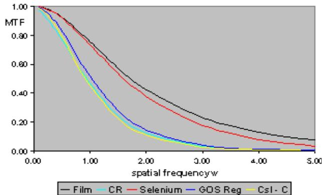
**Fig 9(b).** Comparison of MTF of Film ,CR and DR systems at Ir-192 energy
