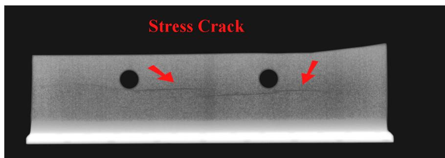
**Fig 12. A sample of Aluminium wing with a stress crack**
