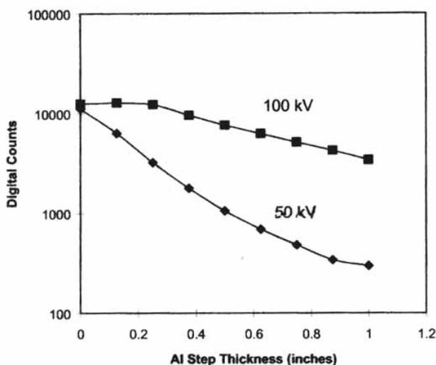
**Fig 7(a) Subject Contrast obtained with a-Se FPD in Aluminium**
