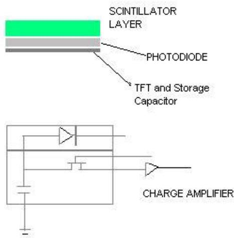
**Fig 3. Structure of an individual pixel and its circuit representation**
