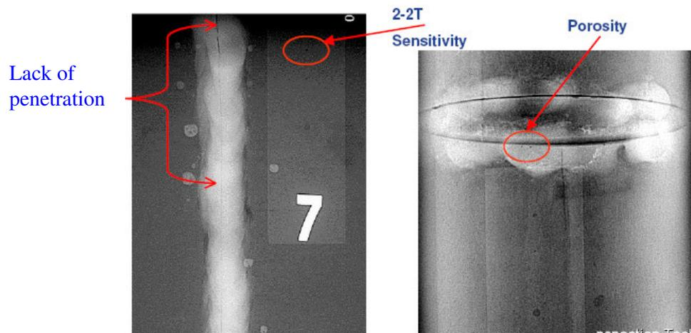
**Fig 11. Weld radiography Images taken by indirect type FPD**
