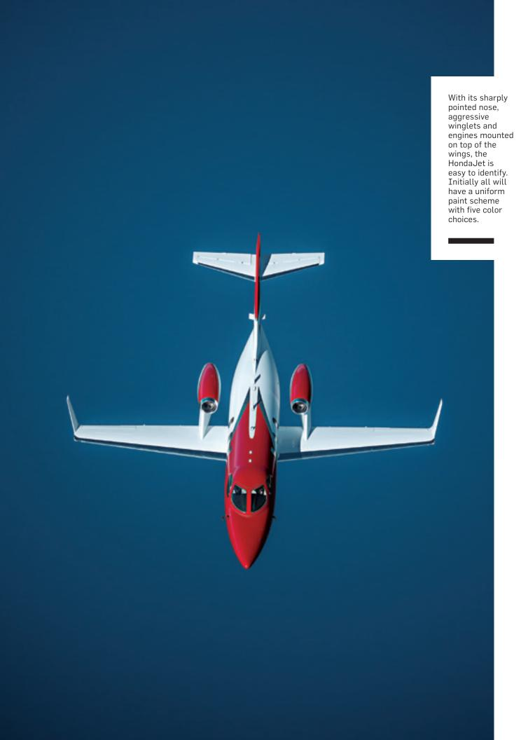
Beyond the vision of producing aircraft under the world-renowned Honda brand, Fujino conceived an overthe-wing mount for the jet engines, claiming the new configuration would provide a quieter cabin and better performance. With the ink now dry on the FAA certification papers, we finally had an opportunity to put this new light twinjet to the test. Could the airplane really do all that Fujino originally envisioned?
