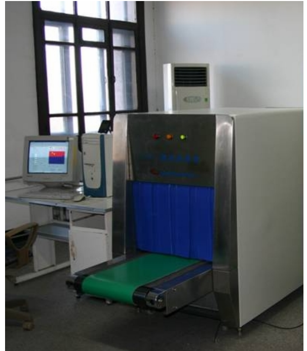
FIG. 8: Laboratory systems of RDX detection with probe volumes of 140 liters.
