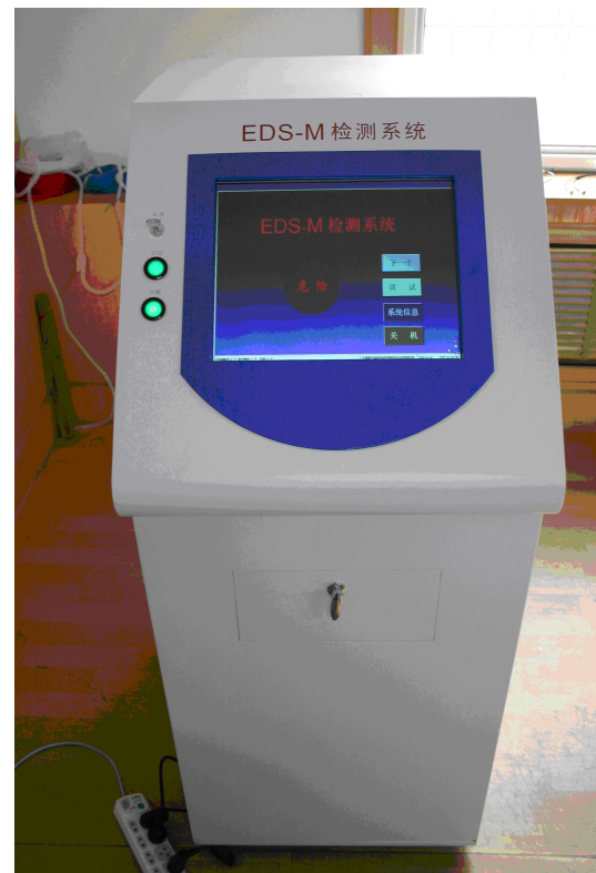
FIG. 9: Laboratory systems of RDX detection with probe volumes of 10 liters.
