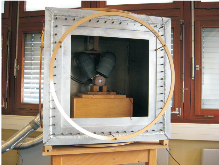
Figure 3.11: Probe head inside the aluminum shielding box
