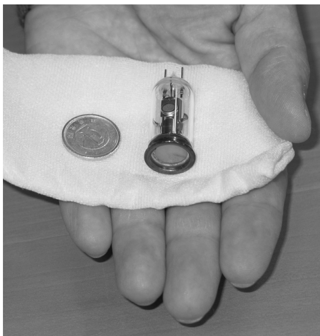
Fig.1 N6601 type transmission type X-ray tube. The diameter of glass is 15 mm. The 1 JPY coin diameter is 20 mm. The direct touch to the X-ray tube is a cause of electric discharge.
