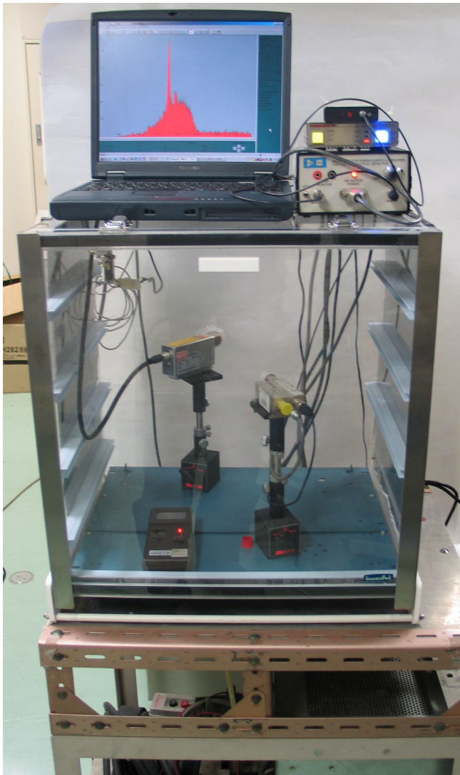
Fig.4 Total view of X-ray fluorescence spectrometer used in the present experiment. Amptek Si-PIN detector (right), X-ray generator (left), survey meter (bottom), and detector controller, X-ray power supply, pulse height analyzer, and computer (top) are shown.
