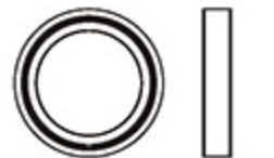
Bearing 輪承 ( \phi 15 \times \phi 21 \times 4 \text{mm} ) \times 2
