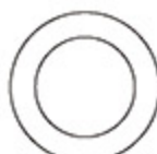
Bearing 軸承 (φ 12x φ 18x4mm) x 2
