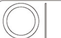
Spacer 單向墊片 \phi 18 \times \phi 22.7 \times 0.7 \text{mm} \times 1
