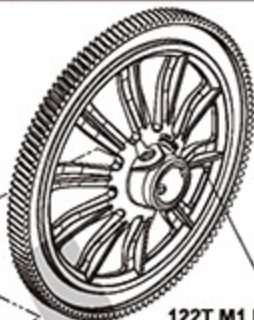
122T M1 Helical Autorotation Tail Drive Gear Set 122T M1 尾驅動斜齒組
