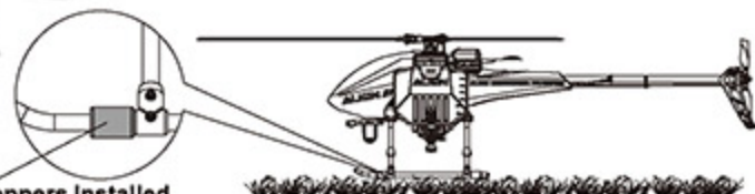
Rubber Skid Stoppers Installed 裝上避震墊圈
