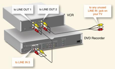
To record your video tapes to a DVD, connect an audio/video cable (not supplied) to the LINE OUT 1 jacks on your VCR to the LINE 3 IN jacks on the recorder. To just watch your video tapes, connect your VCR's LINE OUT 2 jacks directly to any unused LINE IN jack on your TV.
