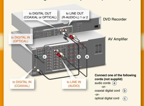
Connecting to an AV amplifier (receiver) with audio cords will enable you to enjoy the TVS surround effects of this recorder, while connecting with digital cords will enable you to listen to Dolby Digital or DTS surround effects. For further explanations, see "Connecting the Audio Cords" in the Operating Instructions.
