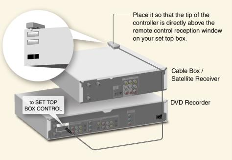
You can have the recorder change the channel of your cable box or satellite receiver to the channel you want to record, just before the timer recording starts. Connect the Set Top Box controller(supplied), and select "Yes" in step 9 of Setup on the next page.
