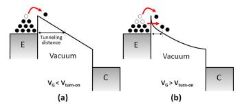
FIG. 3. Energy band diagram of the vacuum channel transistor for (a)  $V_G\!<\!V_{turn\text{-}on}$  and (b)  $V_G\!>\!V_{turn\text{-}on}$ .
