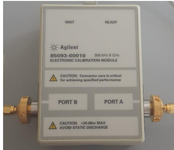
Figure 5.3-1 Electronic calibration module Agilent/HP 85093C, utilized for calibrating vector network analyzer
