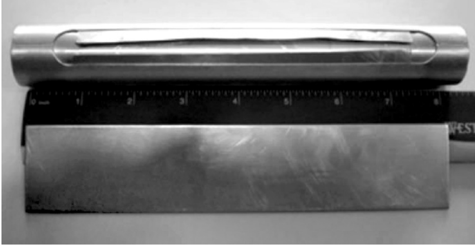
Figure 13. LEU (top) and HEU (bottom) targets for Molybdenum-99 production. These targets would produce the same amount of Mo-99 under the same irradiation conditions. Part of the outer aluminum layer of the LEU target (top) has been removed to show the nickel-coated LEU foil wrapped around an inner aluminum tube. Both targets contain about 5 grams of uranium-235. The LEU enrichment is 19.75 percent. Source: IAEA. 168
