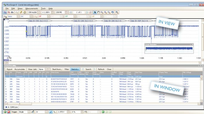
The PicoScope 3000 Series, with its deep memory, is ideal for serial decoding as it can capture thousands of frames of uninterrupted data. Protocols currently included are I<sup>2</sup>C, I<sup>2</sup>S, SPI, RS232/UART, CAN, LIN and FlexRay. Expect this list to grow with free software updates.
