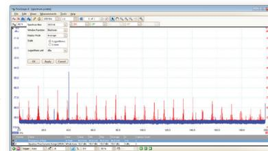
You can display multiple spectrum views with different channel selections and zoom factors, and see these alongside time-domain waveforms of the same data. A comprehensive set of automatic frequency-domain measurements, including THD, THD+N, SNR, SINAD and IMD, can be added to the display.
