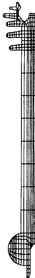
FIG. 2.16. Combustion instabilities: grid of a motor cavity for calculation of acoustic modes.
