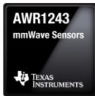
AWR1243: High performance radar front end
