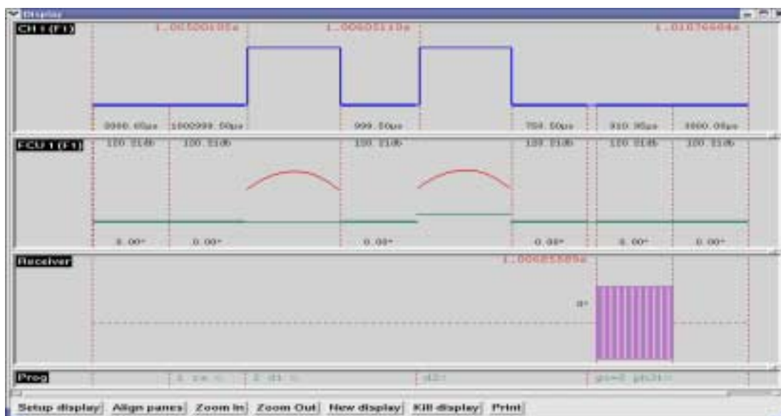
Figure 12. Screen capture of the spin echo pulse program for one cycle using the plusdisp utility within xwinnmr . The pulse width, power, and shape parameters as well as delay times are shown.
