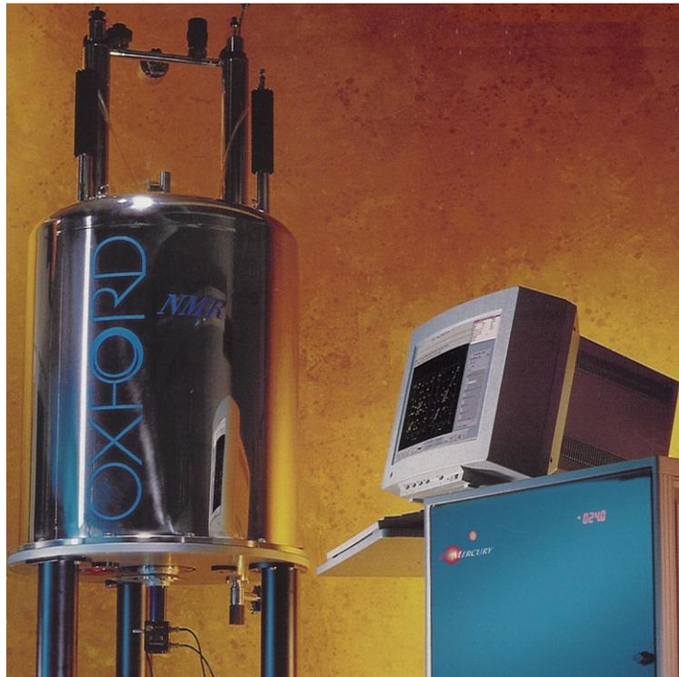
**FIGURE 1.3.1** A commercial NMR spectrometer used for spectroscopy and now, quantum computing.
