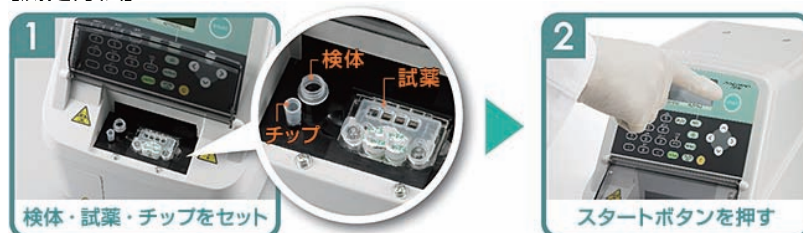
Fig. 2 Quantitative immunoassay system for the measurement of TSH and COR in dog serum.
