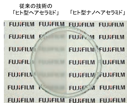
Fig. 7 Comparison of the transparency of "nano hair ceramide" and conventional hair ceramide preparation
