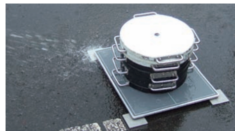
Fig. 6 Waterproof test under load pressure (100 kgf)
