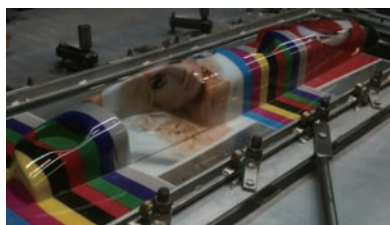
Fig. 5 Examples of a vacuum-forming product digitally molded by an UV inkjet ink (KV). These examples show trial productions of the dashboard of a car (left) and of a three-dimensional signboard used at stores and other commercial facilities.
