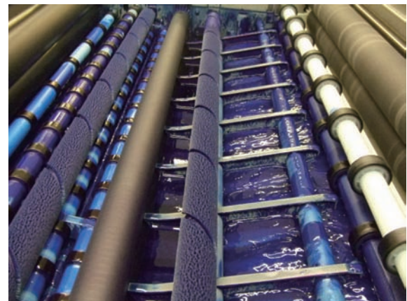
Fig. 3 Precipitation in a present developer tank
