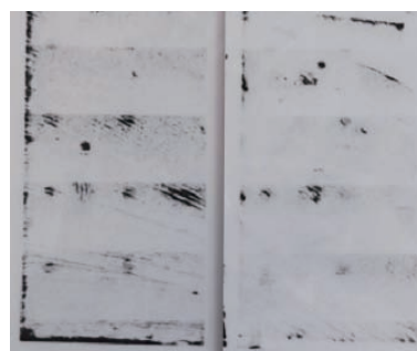
Fig. 7 Example of blocking. After printing, the print side and the backside were placed on top of each other. After storing for 24 hours, blocking occurred in which an ink film (black) became attached to the backside (white matrix).
