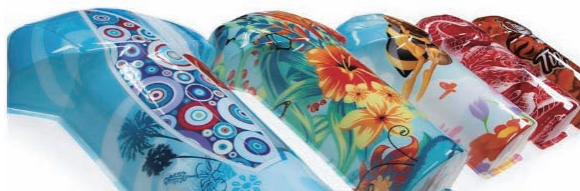
Fig. 5 Examples of a vacuum-forming product digitally molded by an UV inkjet ink (KV). These examples show trial productions of the dashboard of a car (left) and of a three-dimensional signboard used at stores and other commercial facilities.
