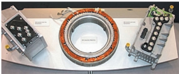
Fig. 8 ISG machine and inverter
