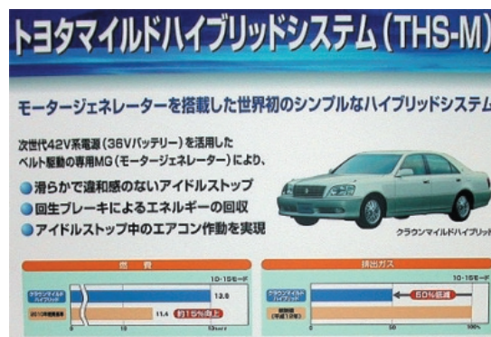
Fig. 4 Toyota Mild Hybrid System
