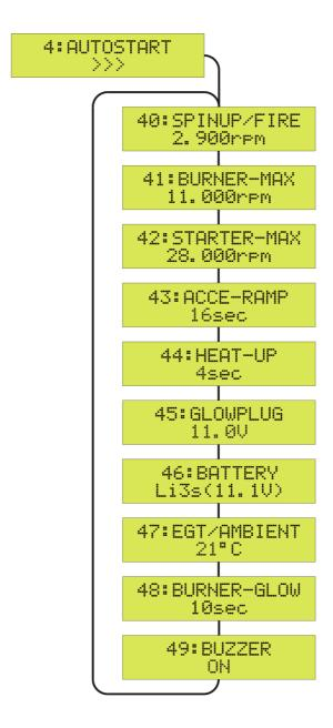
To quit the 4:AUTOSTART menu and to return to the SETUP menu, press the SET key for more than 2 seconds (ESC).
