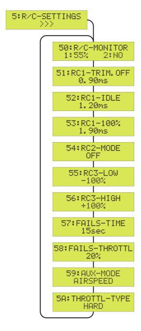
To quit the 5:R/C-SETTINGS menu and to return to the SETUP menu, press the SET key for more than 2 seconds (ESC).
