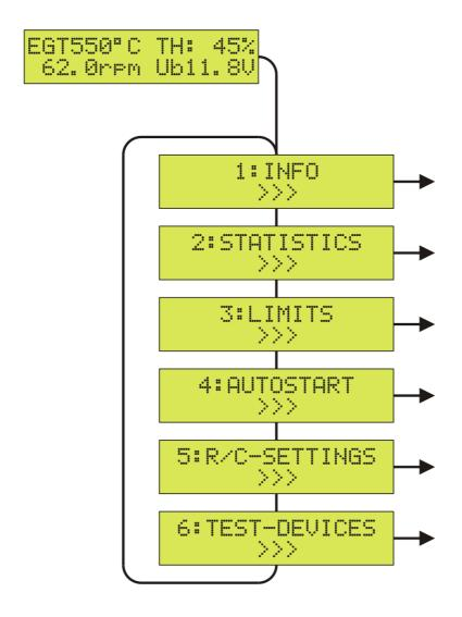
To quit the SETUP menu and to return to the operating status display, press the SET key for more than 2 seconds (ESC). In the following, the individual submenus of the SETUP menu are described.
