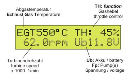
THE = Throttle is a combined function display and error display for the engine operation.
