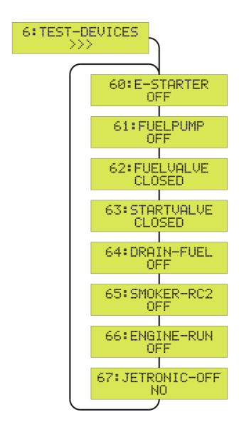
To quit the 6:TEST-DEVICES menu and to return to the SETUP menu, press the SET key for more than 2 seconds (ESC).
