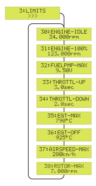
To quit the 3:LIMITS menu and to return to the SETUP menu, press the SET key for more than 2 seconds (ESC).
