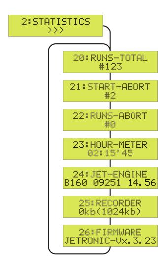
To quit the 2:STATISTICS menu and to return to the SETUP menu, press the SET key for more than 2 seconds (ESC).
