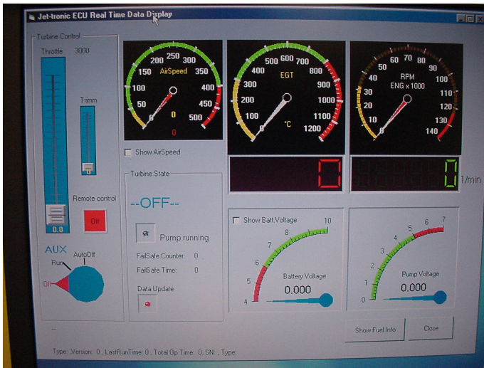
Fig. 1. Jettronic for Windows software used to control the jet turbine
