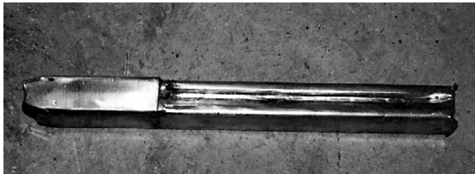
Upper jacket in place on magazine body.
