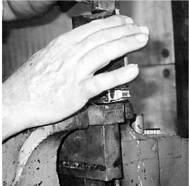
Rear sides are folded and formed using hammer and swage.
