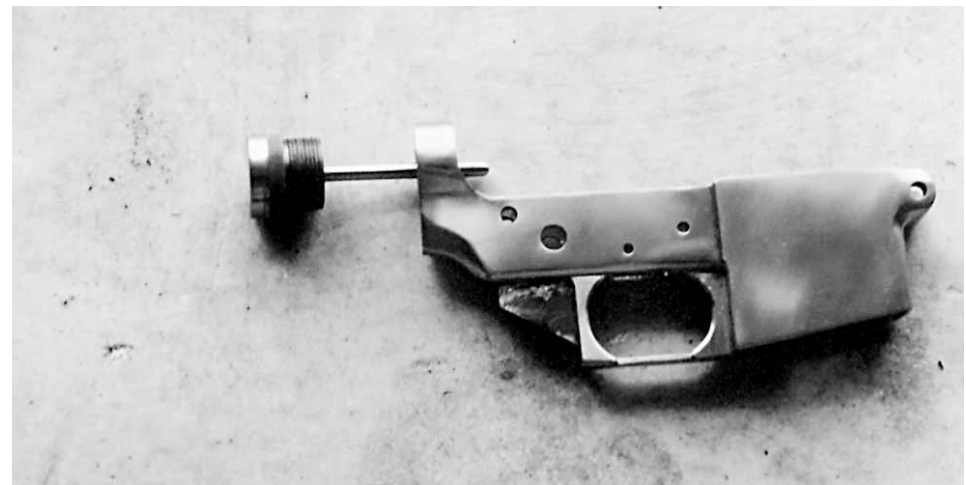
Lower receiver with open bolt plug partially inserted.
