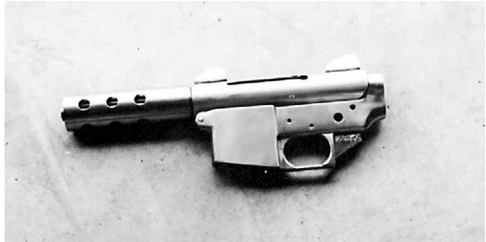
Completed lower receiver with pistol version upper pinned in place.
