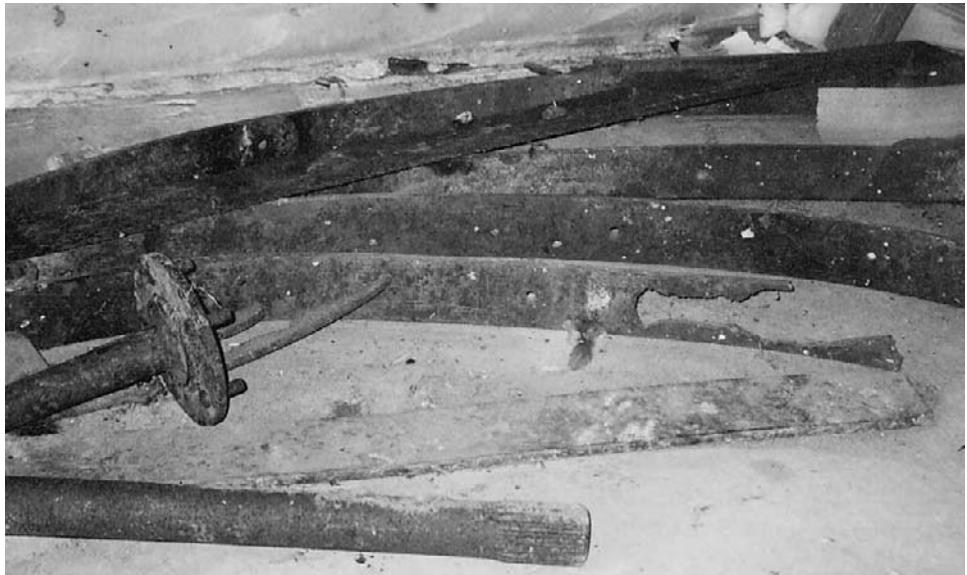
Leaf springs are the source of heat-treatable flat stock.
