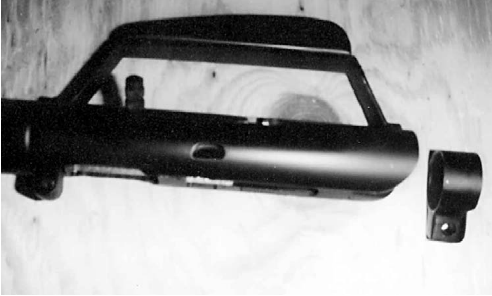
Cut near center to clear bolt release.
