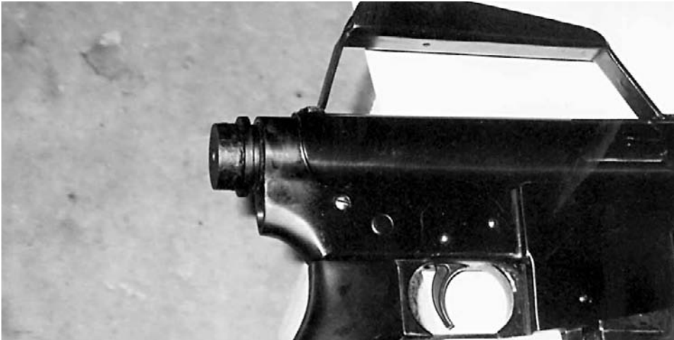
Breech plug partially screwed in place.
