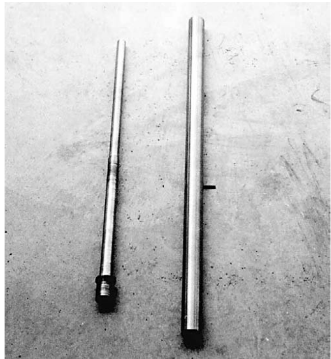
Rifle barrel shown with unturned blank.
