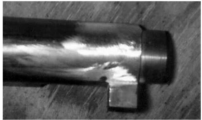
Welds are dressed flush with the surface.
