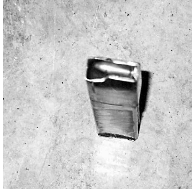
Magazine with cartridge in place, ready for feeding.
