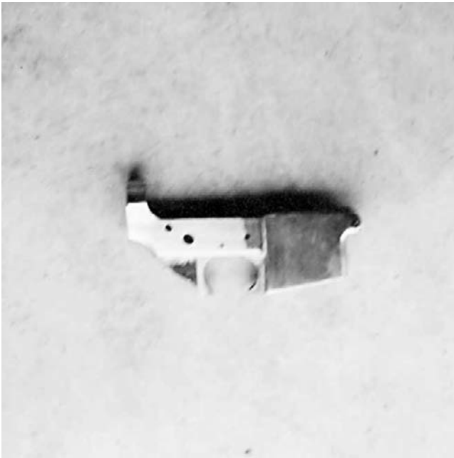
Rear guard welded in place.
