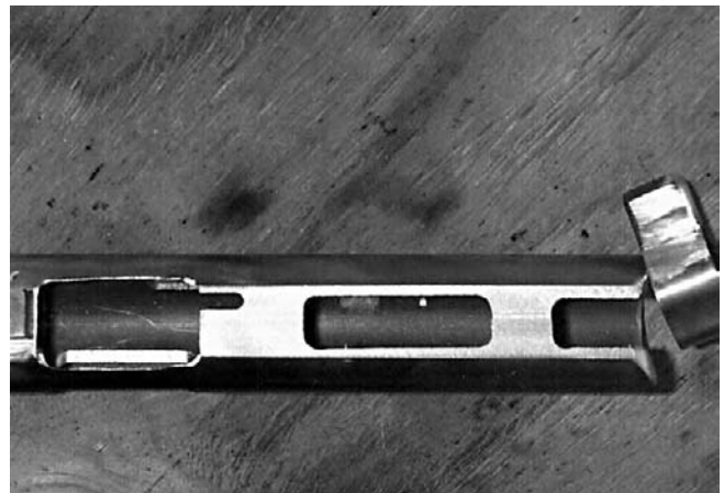
Various openings are formed as required.
