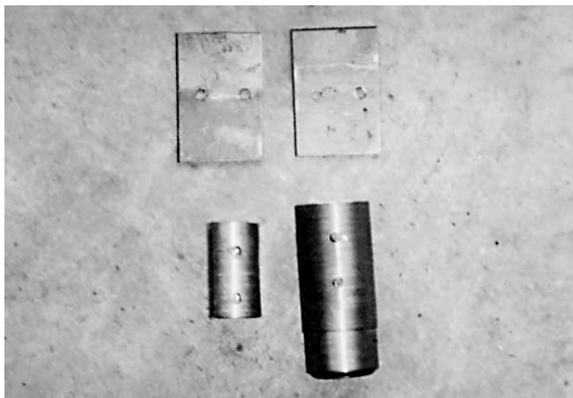
Pistol sight blanks shown with form die.
