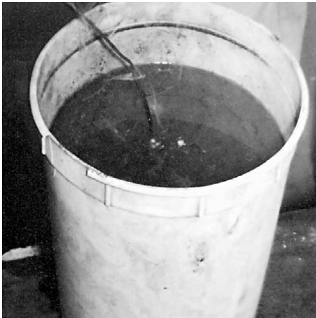
. . . and quenched when desired color (usually bright cherry red) is reached.
