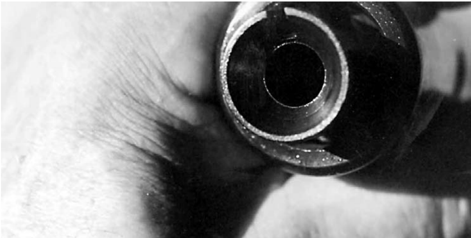
Breech end of barrel, showing approach cone.
