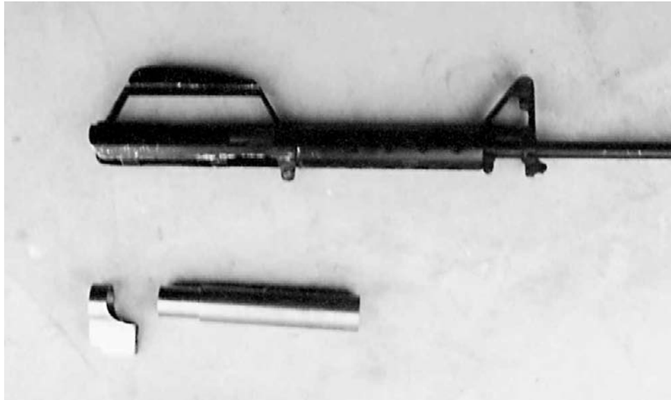
Mandrel is used to align parts for welding.
