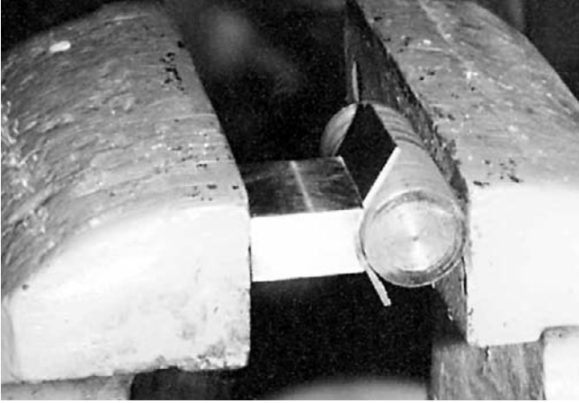
Formed to shape in vise.
