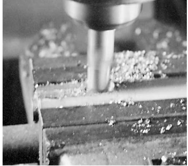
Magazine clearance is cut with end mill.
