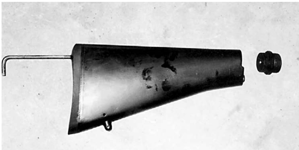
Surplus M16 butt stock is mounted using through bolt and brech plug adaptor. Recoil pad is added for extra length.
