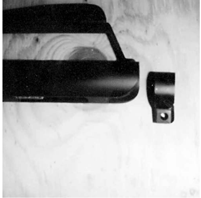
Rear receiver-mounting bracket.
