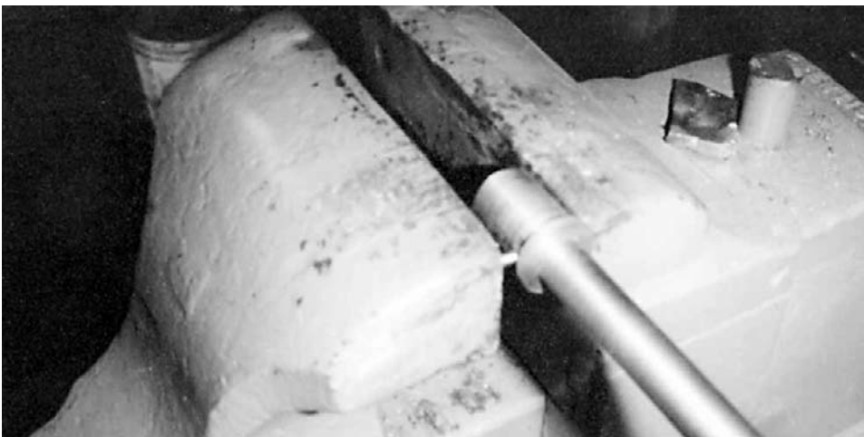
Indexing pin is pressed in place using vise jaws.
