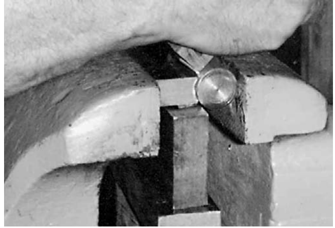
Sides are folded over with hammer.
