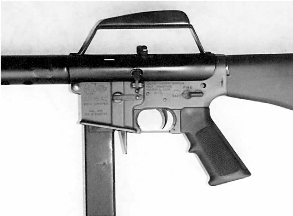
9mm conversion unit mounted on commercial receiver.
