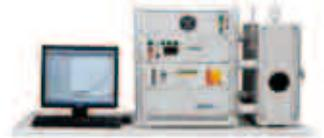
\* **3T 高温超電導磁石オプション – High- $T_c$  cryogen-free superconducting magnets for high field relaxometry:** Manufactured by HTS-110; Extends the NMR field range up to 3 tesla either in combination with Spinmaster or SMARTracer™.
