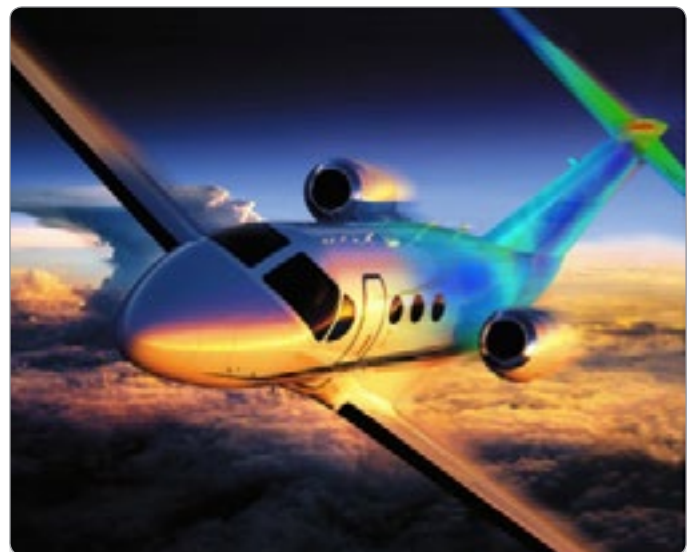
Figure 1: Cessna 510 Citation Mustang* designed and analyzed using NEi Nastran*. Colors superimposed on the empennage indicate levels of stress in the structure. The red end of the spectrum is used for higher values versus blue for lower values.
