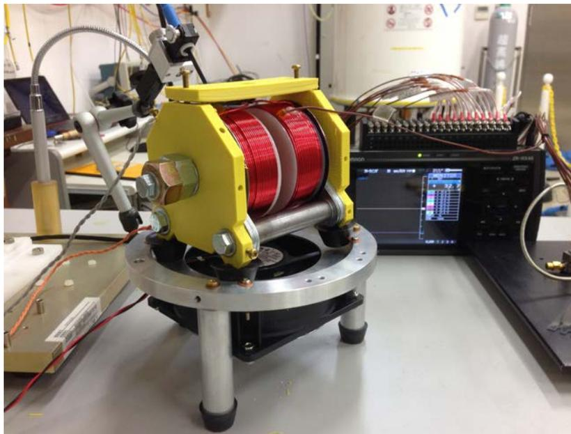
Partially 3D-printed electromagnet
