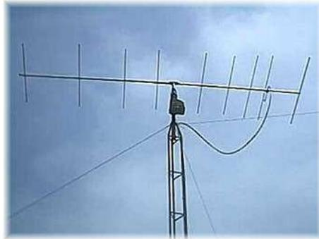
**Figure 7.** Yagi antenna array.
