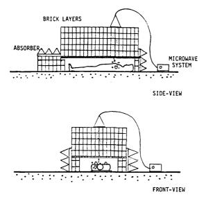
Fig. 4. Experimental step for the measurement of heart and breathing signals of a human subject under layers of bricks using the microwave lifedetection system.
