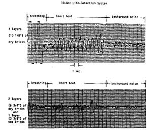
Fig. 8. Heart and breathing signals of a human subject measured through walls of dry and wet bricks with the 10-GHz microwave life-detection system. One layer of wet bricks severely hampered the penetration of the microwave beam.
