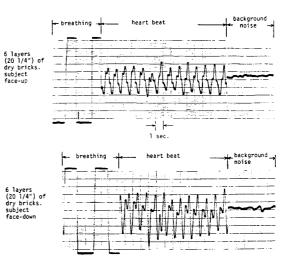
Fig. 6. Heart and breathing signals of a human subject, lying with face-up or face-down position under six layers of bricks, measured by the 2-GHz microwave life-detection system.
