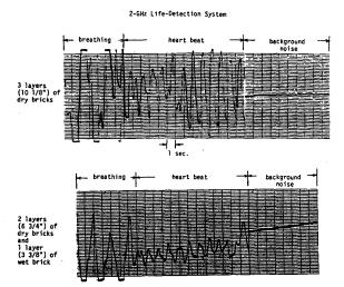
Fig. 9. Heart and breathing signals of a human subject measured through walls of dry and wet bricks with the 2-GHz microwave life-detection system. One layer of wet bricks had a considerable but not severely hampering effect on the penetration of the microwave beam.
