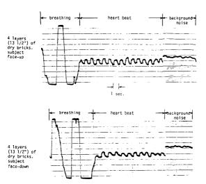
Fig. 5. Heart and breathing signals of a human subject, lying with face-up or face-down position under four layers of bricks, measured by the 10-GHz microwave life-detection system.
