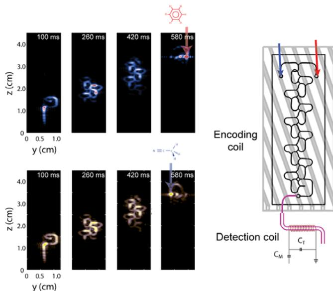
**Figure 1.** TOF partial images of fluid flow through a lab-on-a-chip device. Information about the spatial origin of each fluid species is encoded and stored along the  $B_0$  axis before stroboscopic acquisition in the detector by a microsolenoid detection coil.
