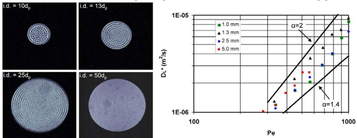
**Fig. 1:** MR images taken with spatial resolution of  $27.3 \mu\text{m}/\text{pixel}$  over an 8 mm thick slice for  $d_p=100 \mu\text{m}$  particles in varying diameter columns. The impact of structural ordering on dispersion dynamics as a function of Peclet number is measured. The lines indicate the Taylor Dispersion  $Pe^2$  and power law fit to data  $Pe^\alpha$  regimes
