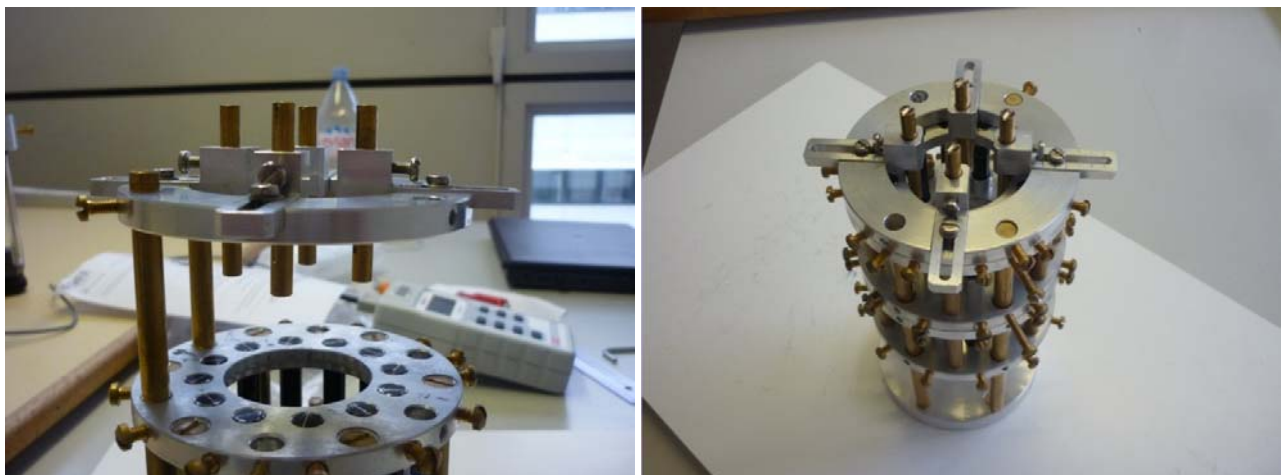
(a) Shim magnets that can move along three degrees of freedom
