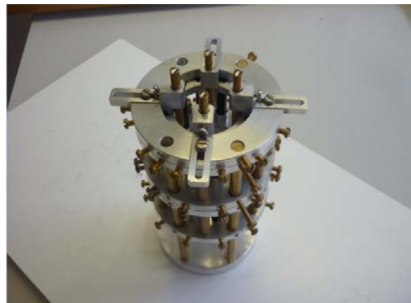
(b) Halbach prototype with the slide-blocks used to move the shim magnets in radial direction.
