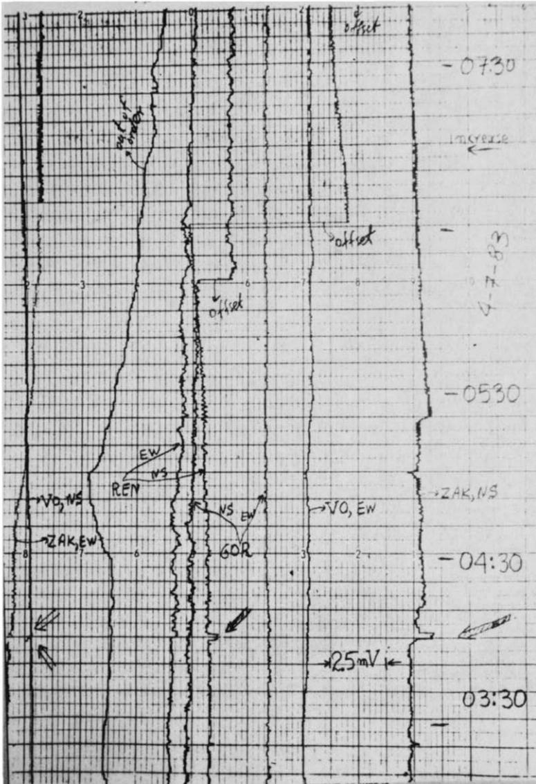
Fig. 7. The simultaneous SES of Fig. 6 recorded at ZAK ( $L_{E-W} = L_{N-S} = 150$  m) and REN ( $L_{E-W} = L_{N-S} = 30$  m). As expected the form of the signal is similar to that of Fig. 6 (the SES on the E-W line of ZAK is seen with some difficulty due to the bad quality of the pen of the recorder). The epicentral distances of ZAK and REN are 610 and 300 km respectively.
