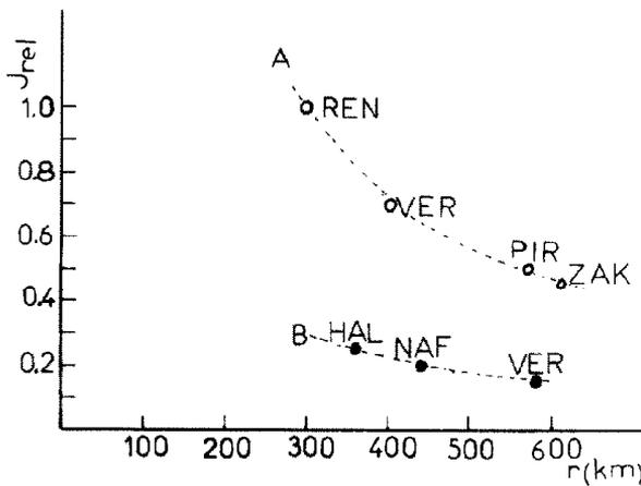
Fig. 14. Signal intensity versus epicentral distance. Curve *A*:  $M = 6.5$  event in the Dardanelles; curve *B*:  $M = 4.5$  event that occurred at 02:39 on June 9, 1983 at  $(37.8^\circ\text{N}, 27.7^\circ\text{E})$ . The lines have been drawn as a visual aid.
