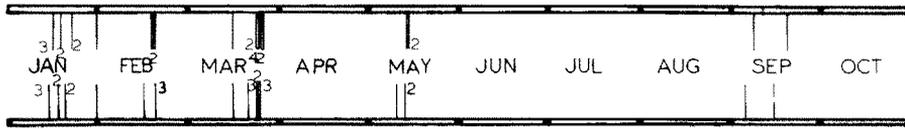
Fig. 1. Time charts of EQ and SES from Jan. to Oct. 1983. Lines above: all EQ with a magnitude greater or equal to 5 that occurred within a radius of 150 km from PIR. Further an  $M = 4.8$  event on Febr. 20, 1983 at a small distance ( $10 \pm 5$  km) from PIR has been included. Lines below: all SES recorded at PIR with  $\Delta V > 0.5$  mV. The numerals give the number of events. The data since Jan. 19 are given in Table 3 (p. 117).
