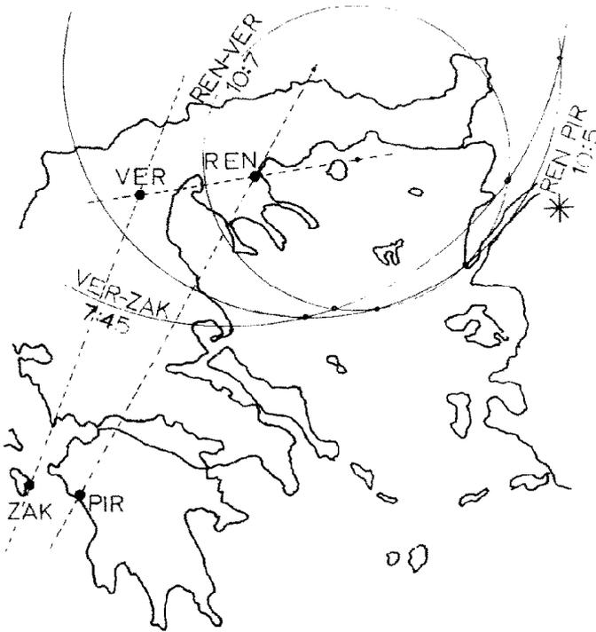
Fig. 13. Graphical determination of the epicenter of the  $M = 6.5$  event that occurred at 12:01, July 5 in the Dardanelles. The SES was recorded at REN, VER, ZAK and PIR. The Apollonian circles correspond to the pairs of stations denoted in the figure. The star shows the true epicenter and solid circles the predicted epicenter from the intersection of the circles.
