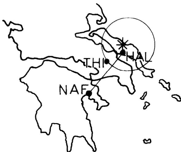
Fig. 11. Graphical determination of the epicenter of an EQ which occurred at 18:54 on May 28, 1983. The Apollonian circle corresponds to the ratio of the intensities of the signal recorded simultaneously at HAL and NAF. The asterisk marks the true epicenter.
