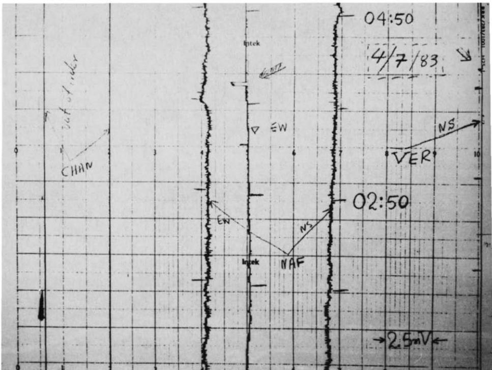
Fig. 9. The same SES as displayed in Figs. 6–8 recorded on the E–W line of VER with a length around 1/3 of that of the parallel line depicted in Fig. 6. A comparison of these two figures indicates that  $\Delta V$  is proportional to  $L$  ( $\Delta V/L = \text{const.}$ ). The SES on the other line, N–S, was unfortunately not recorded since the pen was not working at the time. This multipen-recorder has no memory.
