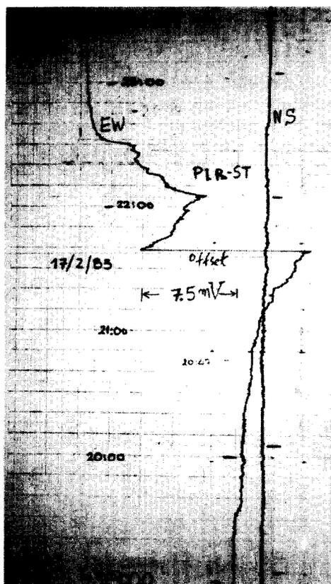
Fig. 4. A strong SES, that belongs to group II, recorded on an E-W line ( $L = 50$  m) at PIR at 20:50, Feb. 17, 1983; it was followed by an  $M = 4.8$ -EQ that occurred at 05:40 on Feb. 20, 1983, with an epicenter close to the station ( $r \approx 10 \pm 5$  km).
