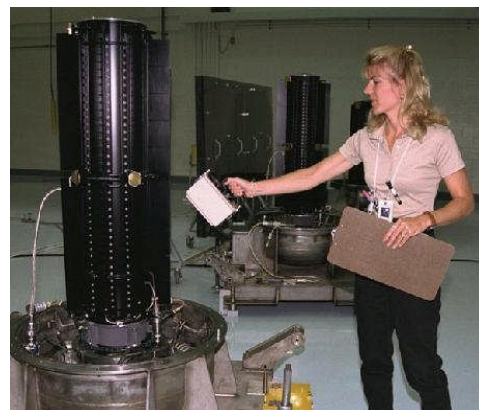
Figura 2.1. NASA Cassini mission General Purpose Heat Source Radioisotope Thermoelectric Generator (GPHS-RTG).
