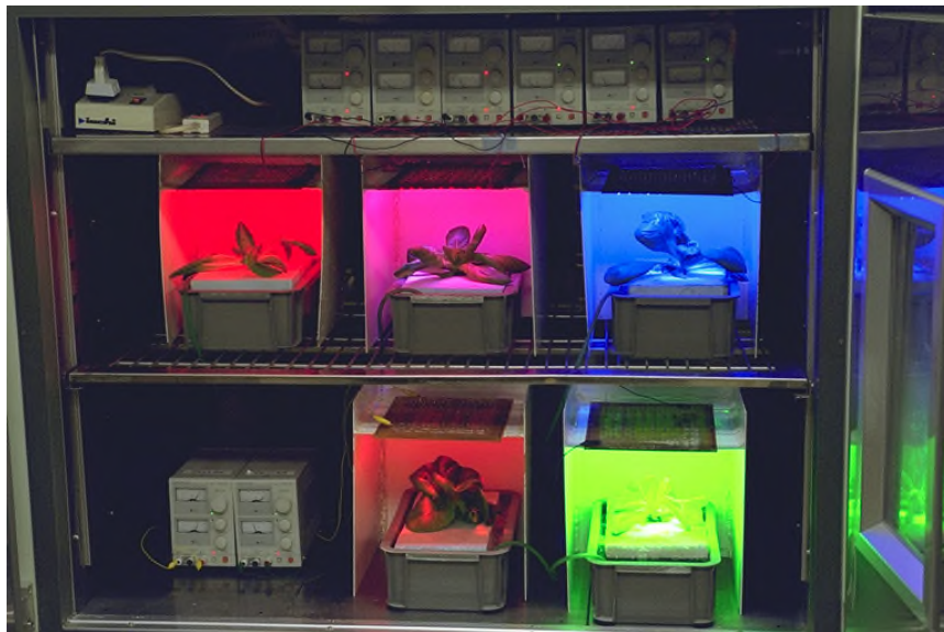
Figure 16.8. Experiments at Tokai University Plant Factory Laboratory growing plants under different colored LED lights. Photo courtesy M. Takatsuji, Dept. of Biology, Science and Technology, Tokai Univ.
