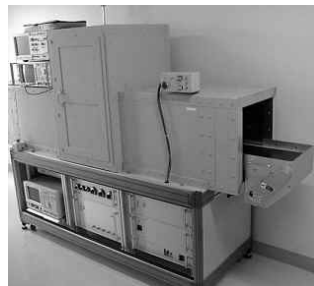
Fig. 11 Prototype of NQR luggage checker developed by the cooperation with Thamway Co., Ltd. in Japan.
