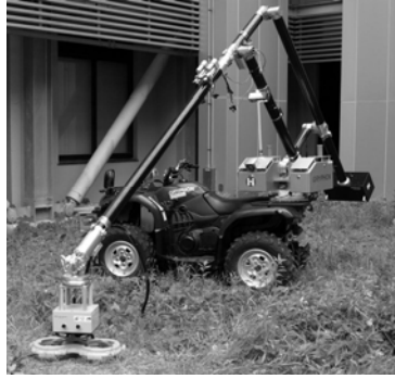
Fig. 10 NQR detector mounted on a mine vehicle developed by Hirose Lab. in Tokyo Institute of Technology [5].
