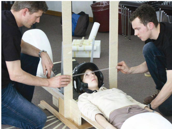
Figure 5-14: Driving position and visibility tests. Measurement of the minimal height of the vehicle body.
