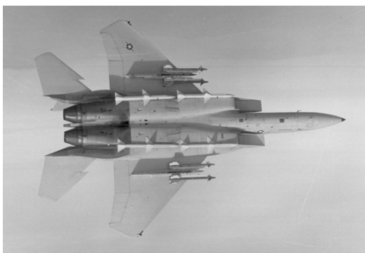
F-15 aircraft flying in steep bank, with four AIM-7s on the fuselage and two AIM-9s on each wing. Official USAF photo.
