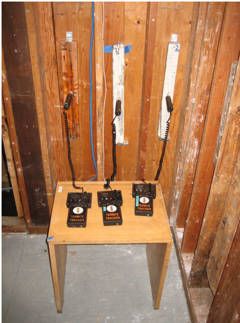
Figure 3. Stud bay 1, wall voids, and AE equipment used to measuring drywood termite feeding activity in field-collected boards. The board in the left hand stud bay is an untreated control board (no termites or damage), middle board has damage only, no termites, and the far right board active with live drywood termites. The black boxes and sensors with flexible cables are for portal AE detection equipment (Tracker, Dunegan Engineering, Midland, TX).
