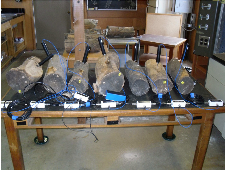
Figure 2. Seven logs from a large Loquat tree ( Eriobotrya japonica (Thunb.) Lindl.) used for the study collected during the summer of 2007 from a private residence in southern California (Granada Hills, CA). The logs were similar in maximum diameter (average 15.1 cm, range 11.4 cm to 19.9), length (average 47.3 cm, range 46.1 cm to 49.0 cm), and age (the homeowner stated the tree was mature, at least 4.5 m in height when cut for firewood in 1998). All logs were placed onto a small wooden table (152.7 cm by 86 cm by 78 cm). To prevent ants (Argentine ant, Linepithema humile (Mayr)) from attacking the logs on the table, the legs of the table were placed into small plastic saucers (15 cm dia by 3 cm deep) containing a 1 cm deep band of motor oil (SAE 30, Ace Hardware Corporation, Oak Brook, IL). Additional ant prevention measures included a applying a 15 cm long band of petroleum jelly (Long Drugs, Walnut Creek, CA) to the cable end leading into the back of main AE Smart controller box. The seven small white boxes (8.9 cm by 3.5 cm by 3.1 cm) seen in the center of the photograph are AE Smart Max-modules (Dunegan Engineering, Midland, TX) and are used in conjunction with software to control the order of sensor selection (randomly) for AE activity during data collection.
