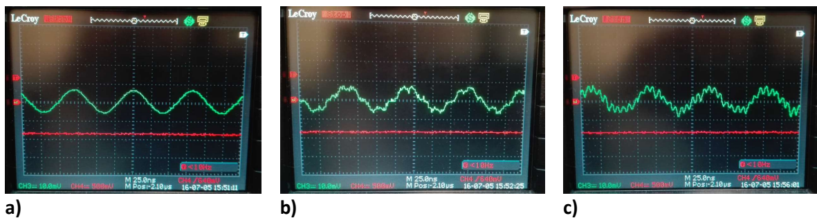
Figure 37 – Measurements of attenuation and noise of a 5mV NMR signal after a) the passive switch, b) the passive switch and the \pi -section and c) the passive switch, the \pi -section and the DC driver connected.
