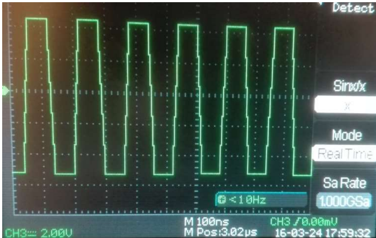
Figure 21 – Saturation of the preamplifier. The preamplifier saturates around 4V with a RF signal at the input of \sim 70\text{mV} .
