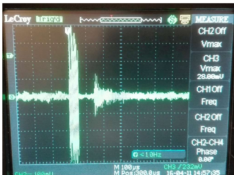
Figure 28 – The first signal is the attenuated RF pulse. The second signal is unexpected behavior, with a decaying shape. This signal appears \sim 100 \mu\text{s} after the RF pulse.
