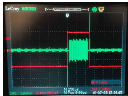
Figure 36 – Attenuation of a RF pulse at 0.3x power and 12.4 MHz (green). The TTL signal is directly measured from the USRP1 (red) 9 .
