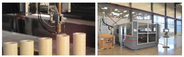
D-DART Fuel Grains Being 3D Printed on the Big Area Additive Manufacturing (BAAM) Machine – Courtesy Cincinnati, Inc.
