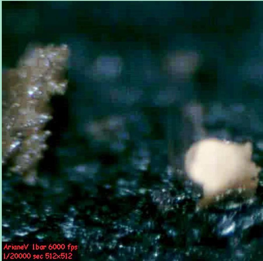
Transition from surface accumulate (skeleton layer) first to aggregates (partial oxidation) and then to agglomerates (burning spheres) for  $\mu\text{Al}$  particle clusters. [Video SPLab: AP/HTPB/ $\mu\text{Al}$  industrial propellant microstructure].
