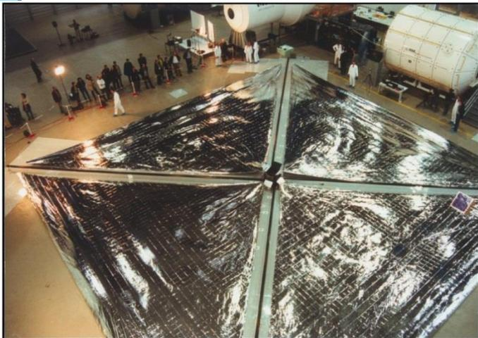
Fully deployed 20 m × 20 m solar sail at DLR-Cologne
