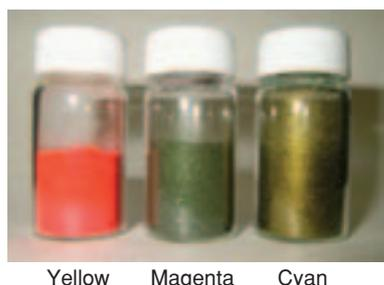
Fig. 2 Appearance of the Fuji dye sets for D2T2 system.
