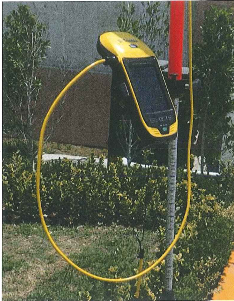
Figure 1 – A Trimble GeoXT Explorer 6000 GPS used to Collect Field Measurements during the FVVGT Visit
