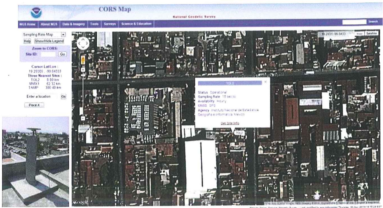
Figure 6 – Location of Toluca CORS Base Station Used to Post Process GCPs
