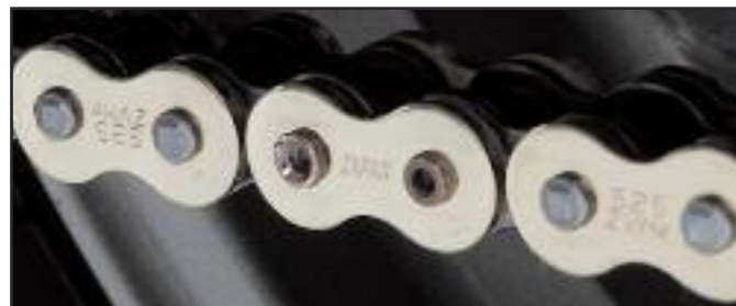
All ZJ rivet style cover plates are press-fit.
